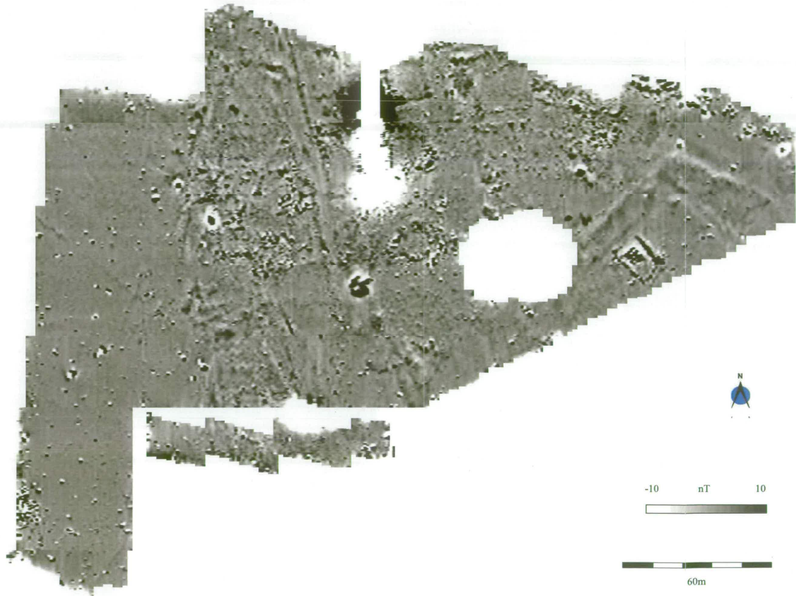
FIG. 2: Gradiometer Survey – Grey scale plot of raw data, scale – 1:1000
