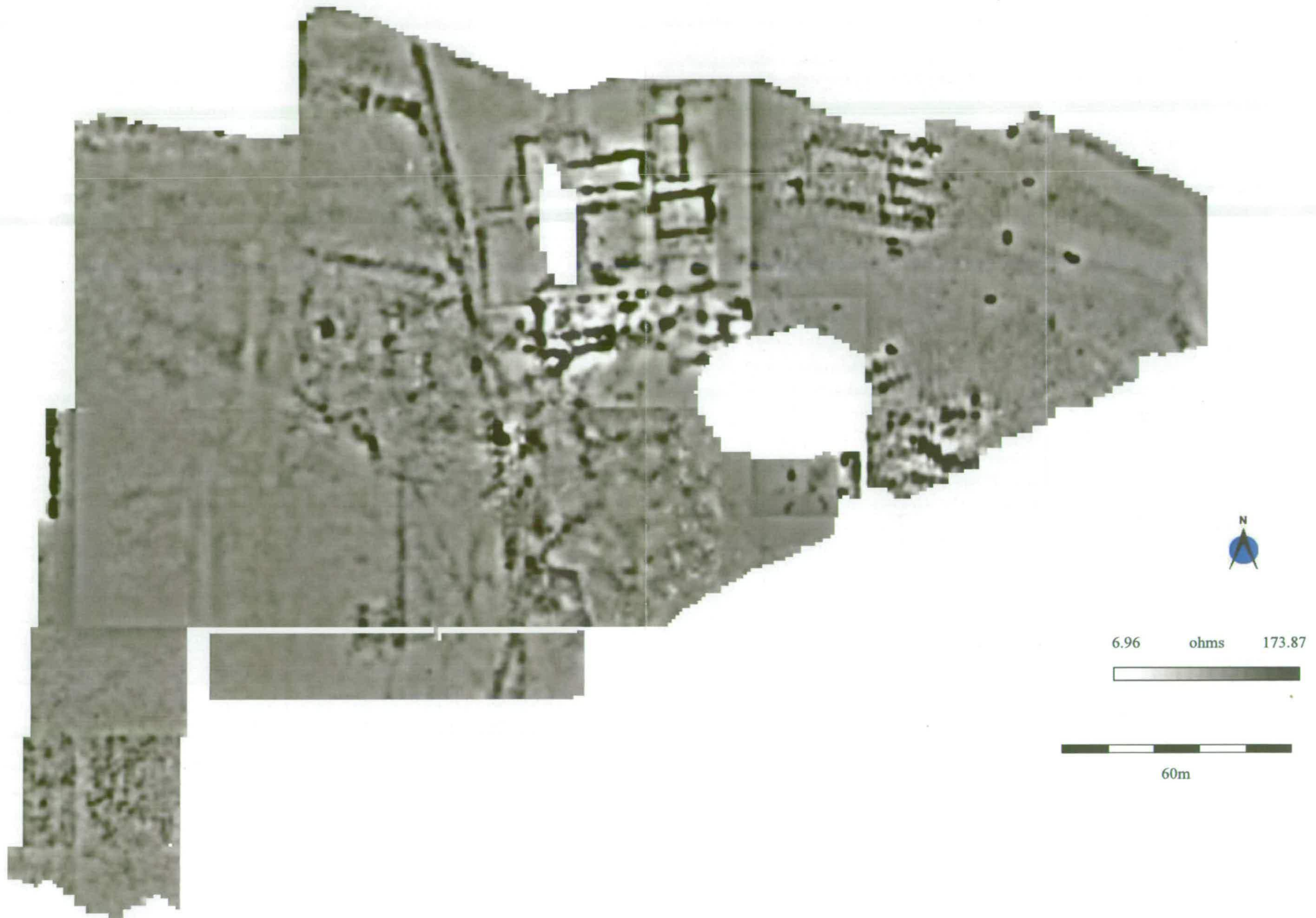
FIG. 8: Earth Resistance Survey – Greyscale plot of enhanced data, scale – 1:1000
