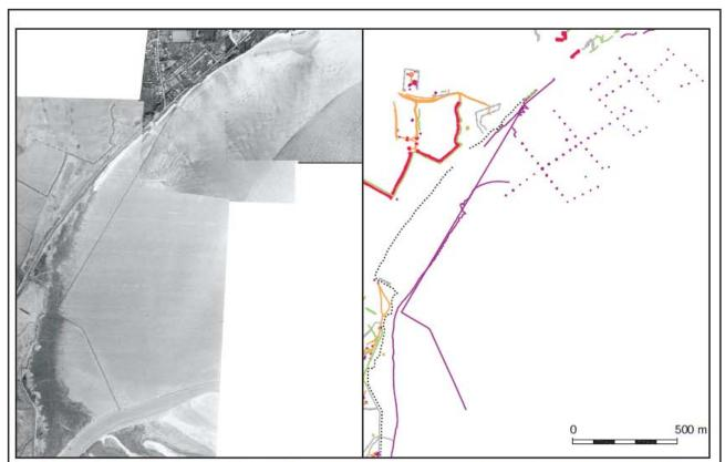
Plate 48. Anti-landing obstacles, Pegwell Bay (MWX43182, MWX43183, MWX43189, MWX43188, MWX43185, MWX43230 and MWX43173). NMR RAF/HLA/540 6052-6053 17-MAY-1942 and NMR RAF/106G/UK/1110 4077 10-JAN-1946 © English Heritage (NMR) RAF Photography
