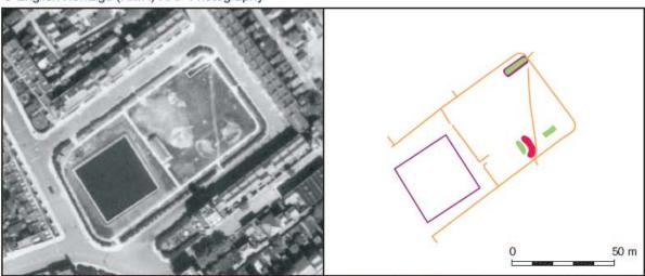
Plate 51. Emergency Water Supply reservoir beside an entrance to the Ramsgate Underground Air Raid Shelter (MWX43112 and MWX43094). NMR RAF/HLA/540 6095 17-MAY-1942 © English Heritage (NMR) RAF Photography
