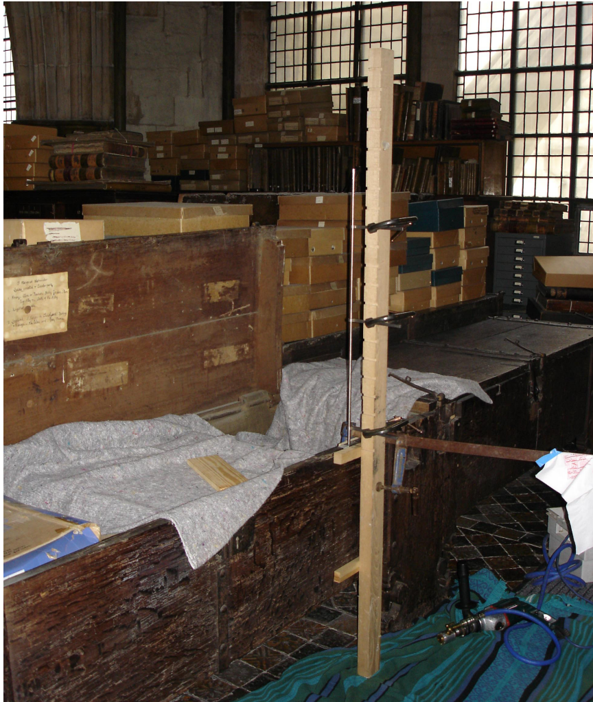
Figure 45: Drilling the Long Chest with the micro-borer (D Miles)
