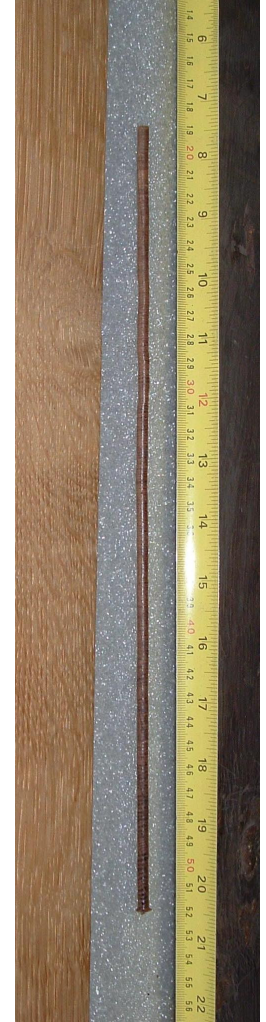
Figure 46: Micro-bore hole (8mm diameter) and core (M Bridge)
