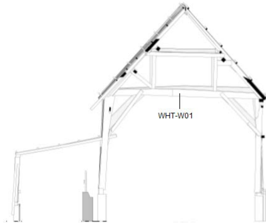
Figure 9: Section through Truss 1, east face, showing the sampled timber, WHT-W01 (after ATD London Ltd)
