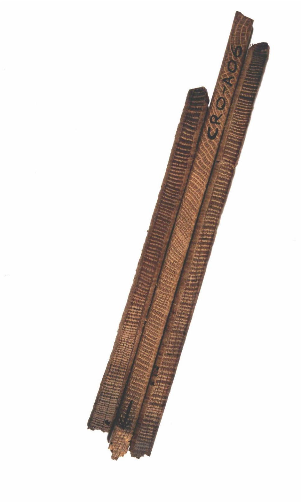
Figure A4: Three cores from timbers in a building. They come from trees growing at the same time. Notice that, although the sequences of widths look similar, they are not identical. This is typical
