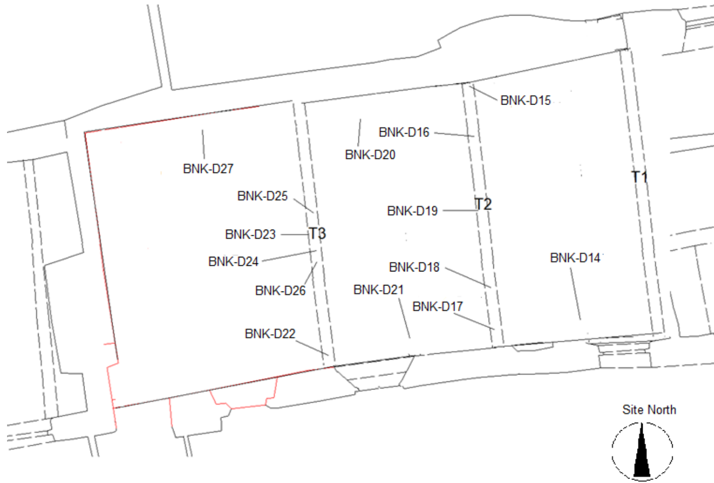
Figure 10: Representative first-floor plan, showing the location of sampled timbers BNK-D14–27 (after Lane, Bayer, and Roethe, Historic England)
