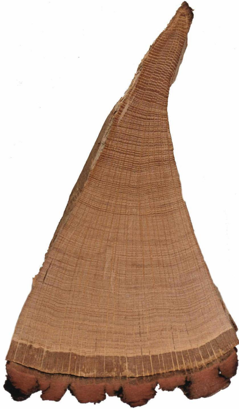
Figure A1: A wedge of oak from a tree felled in 1976. It shows the annual growth rings, one for each year from the innermost ring to the last ring on the outside, just inside the bark. The year of each ring can be determined by counting back from the outside ring, which grew in 1976
