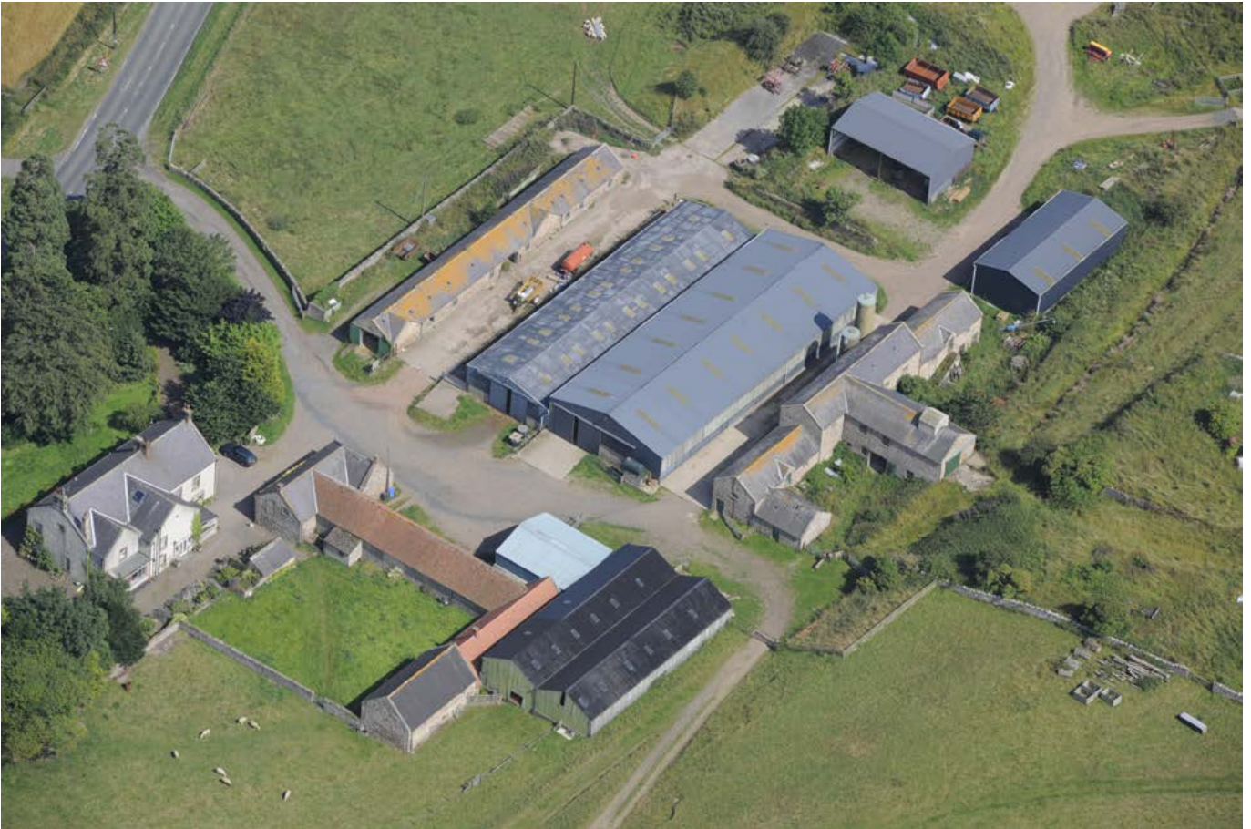
Farmstead at Humbleton. Modern sheds have been placed within the large cattle yard, note the T-shaped barn and mixing house range which is characteristic of larger farmsteads in this area. Photo © Historic England 28567/48
