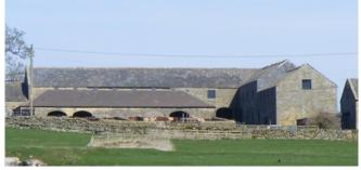
Hemmels – a form of open-fronted shed for fatstock with a small yard – are frequently situated in yards or as in this case sit on the perimeter of a yard. Here the hemmel is divided into two separate areas, each with two arched entries accessing two small, stone-walled enclosures. Photo © Jen Deadman
