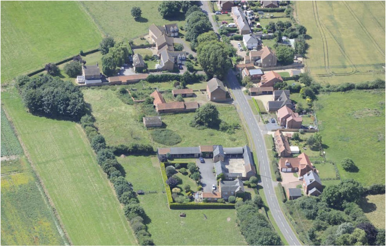
Farmsteads in the medieval settlement of Swaton were all rebuilt in the early to mid-19th century, with barns, stables with granaries and shelter sheds to regular courtyard layouts. Note the hedged boundaries to the earlier plots, contrasting with the typical fenland enclosures bounded by ditches. Photo © Historic England 28554/056
