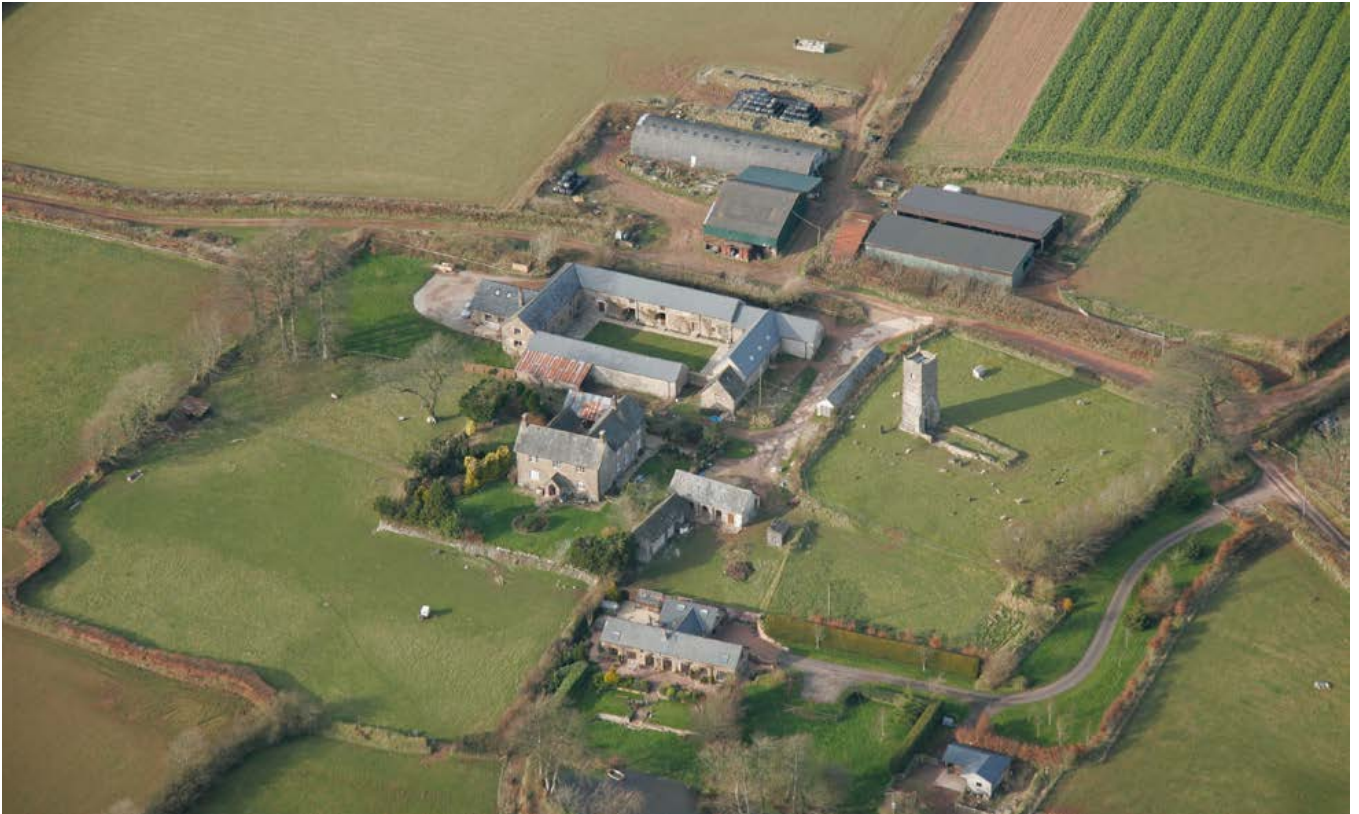
This regular courtyard farmstead at Upton developed next to the long-derelict 14th-century church. It results from a comprehensive scheme of rebuilding in about 1860, and is typical of the largest-scale courtyard plans of this type in having separate access to the farmhouse which enjoys views looking away from the farmyard over its own garden. Photo © Historic England 23829/003
