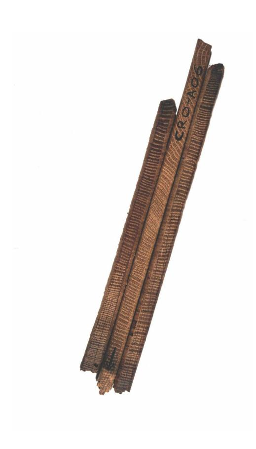
Figure A4: Three cores from timbers in a building. They come from trees growing at the same time. Notice that, although the sequences of widths look similar, they are not identical. This is typical
