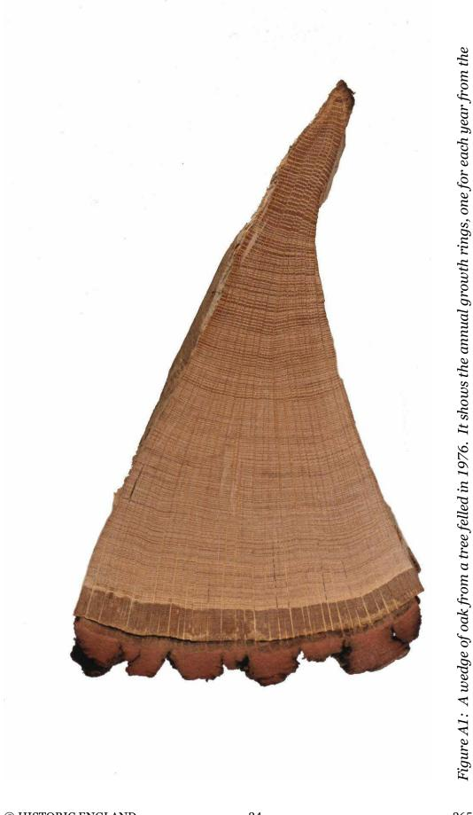
innermost ring to the last ring on the outside just inside the bark. The year of each ring can be determined by counting back from the outside ring, which grew in 1976
