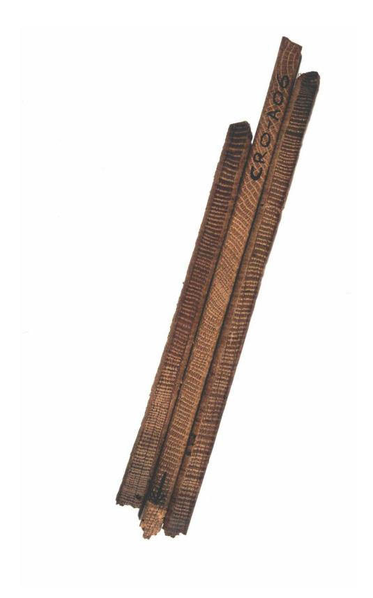
Figure A4: Three cores from timbers in a building. They come from trees growing at the same time. Notice that, although the sequences of widths look similar, they are not identical. This is typical
