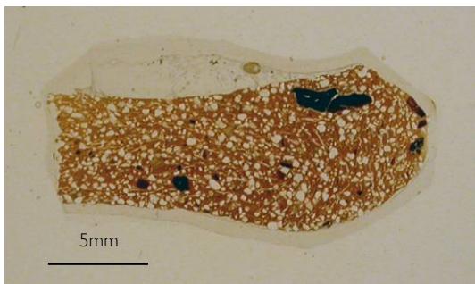
Fig 9: Flaxengate: Thin section of rim of sandy glass-working crucible (F76 P10), cf Figures 7, 38 and 11.
