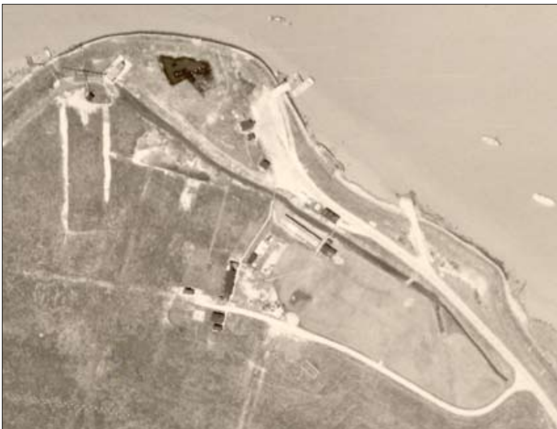
Figure 6: The jetty area in May 1952, at the centre is the long rectangular radar building with SCR 584 radar trailers to either end and a third trailer to the left. RAF58/877 5164 21 May 1952 English Heritage (NMR) RAF Photography
