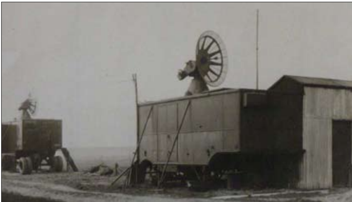
Figure 7: Early 1950s radar station used during the bomb ballistics trials showing two SCR 584 type radars TNA:PRO AVIA 6/14752
