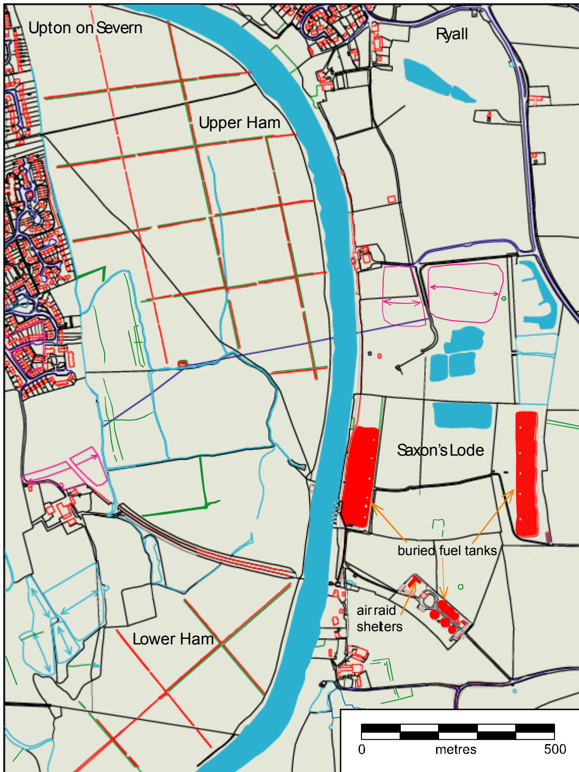
Figure 20: Aircraft obstructions and the fuel store at Saxon's Lode The pattern of red grids across the Hams and Uckinghall meadow are formed by the spoil banks of the aircraft obstruction ditches. The base map is: © Crown Copyright. All rights reserved. English Heritage 100019088, 2009
