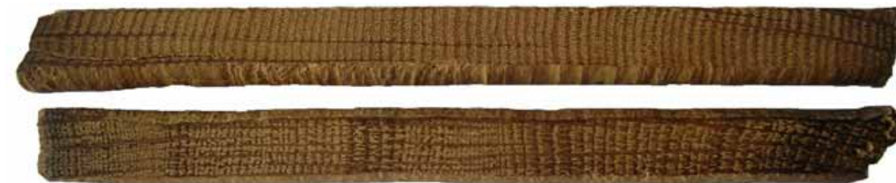
Figure 19: Superficially the samples fell into two groups, the first (upper sample) where the growth rings appeared to be more regular and generally evenly spaced and the second (lower sample) where they were more varied
