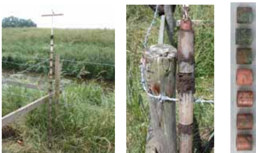
Figure 2 Copper rod removed after 30 months burial. The image on the far right shows the copper samples from the top of the soil profile (0.5m depth) through to the bottom of the profile (1.7m depth)
