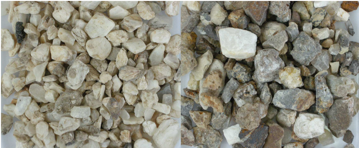
Figure 9: The 5mm to 16mm fraction of sample 36 (left) and sample 37 on the right at the same scale; sample 36 is predominantly barytes, with very little gangue, whereas sample 37 contains a considerable amount of gangue, including fluorspar (amber), limestone (grey) and iron-rich stone (dark brown / orange).
