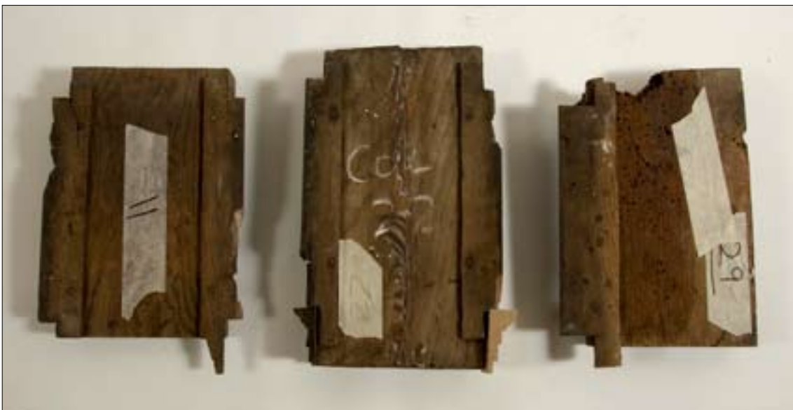
Figure 31. Rear of masks with nailed-on side mouldings.
