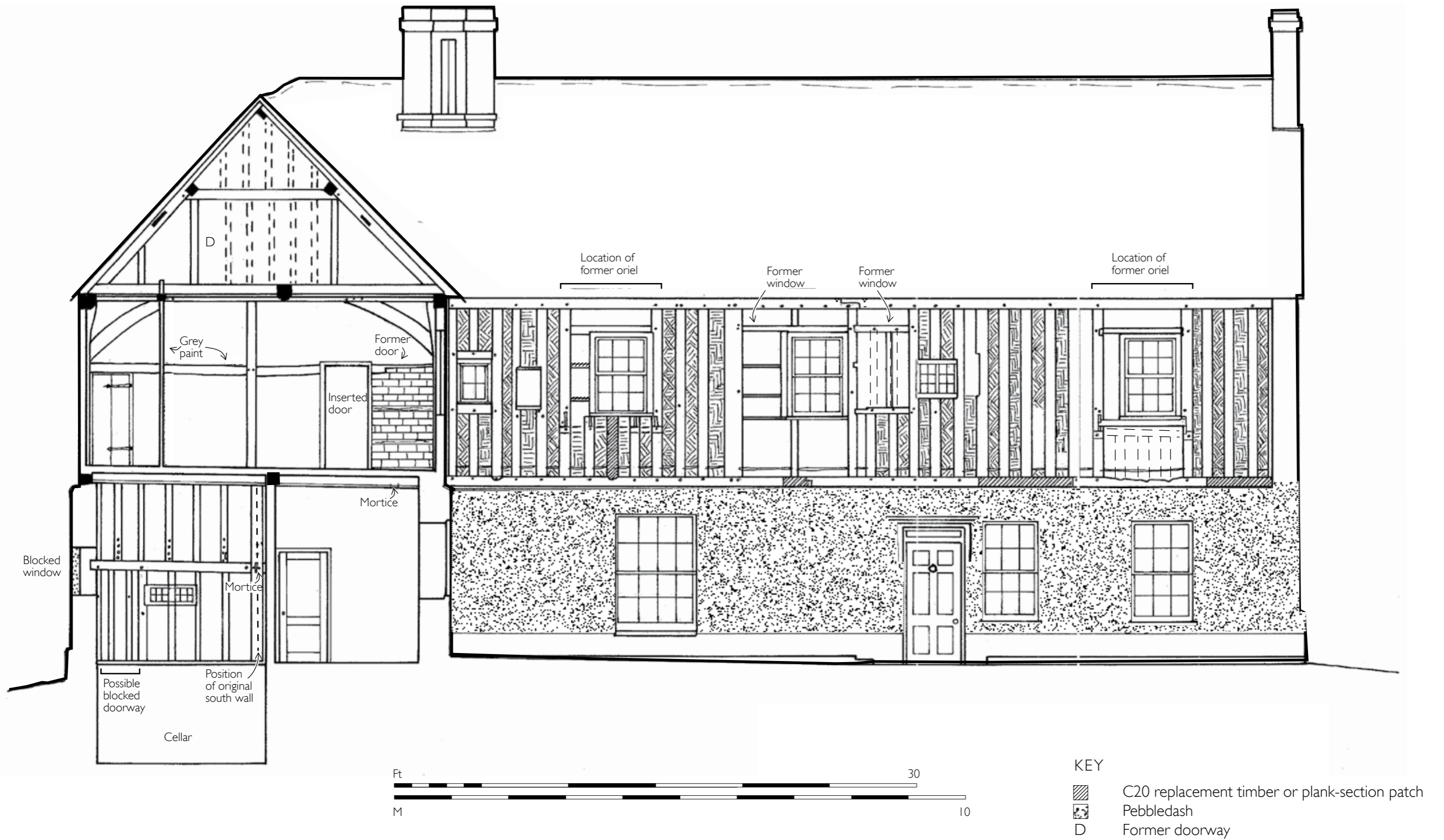
Fig. 71: West elevation of hall range, with cross section of cross wing. (Drawing by Linda Hall; © English Heritage).
