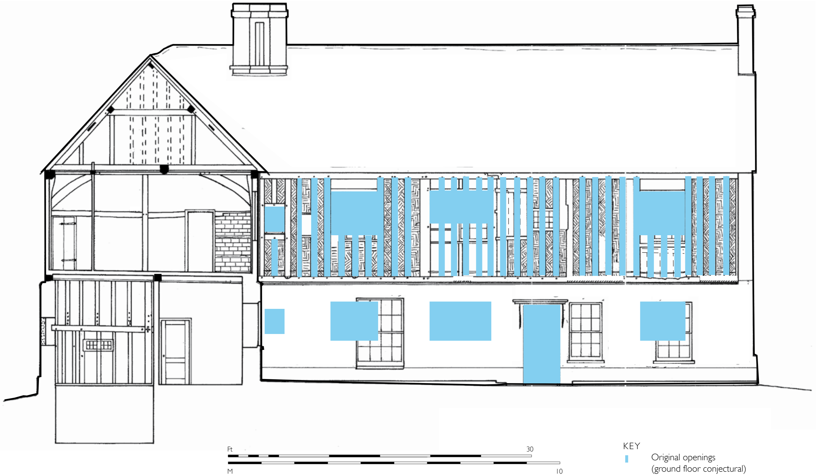
Fig. 72: West elevation of hall range, with cross section of cross wing. Conjectural reconstruction of original window openings shown in blue. (Drawing by Linda Hall; © English Heritage).
