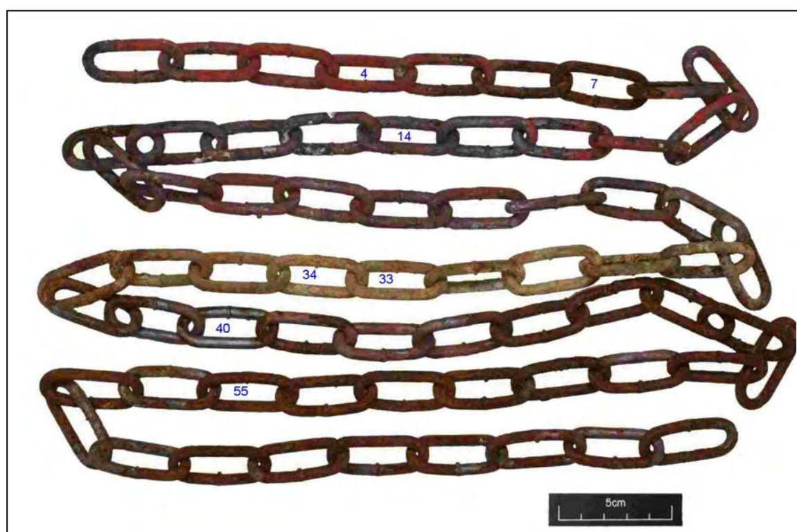
Figure 3. Chain 177, numbered at the links where samples of surface layers were removed for XRD analysis.
