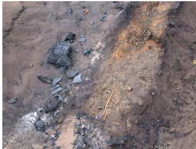
Figure 12 Unburnt soil from beneath a beam (where iron in the soil has not been oxidised).
