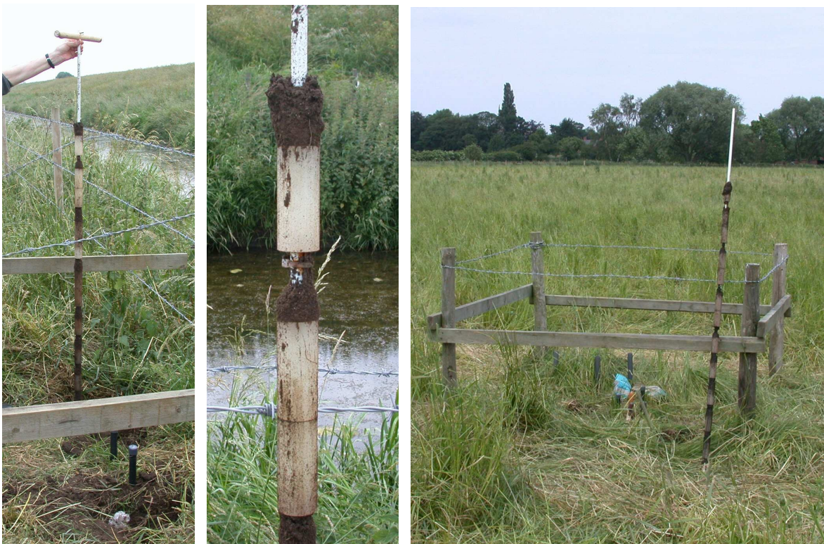
Figure 1. Inert plastic rods bearing iron coupons as recovered after 30 months burial. The iron coupons or bars of c. 50mm length are tied to the rods between the white spacers and are partly hidden in these images by soil that is in the recesses. Left : Rod 4 of Cluster 1 being pulled from the ground. Centre : upper part of Rod 4 of Cluster 1 (the north delph of the River Witham is visible in the background). Right : Rod 4 of Cluster 2 shown leaning against the fencing surrounding the groundwater monitoring point
