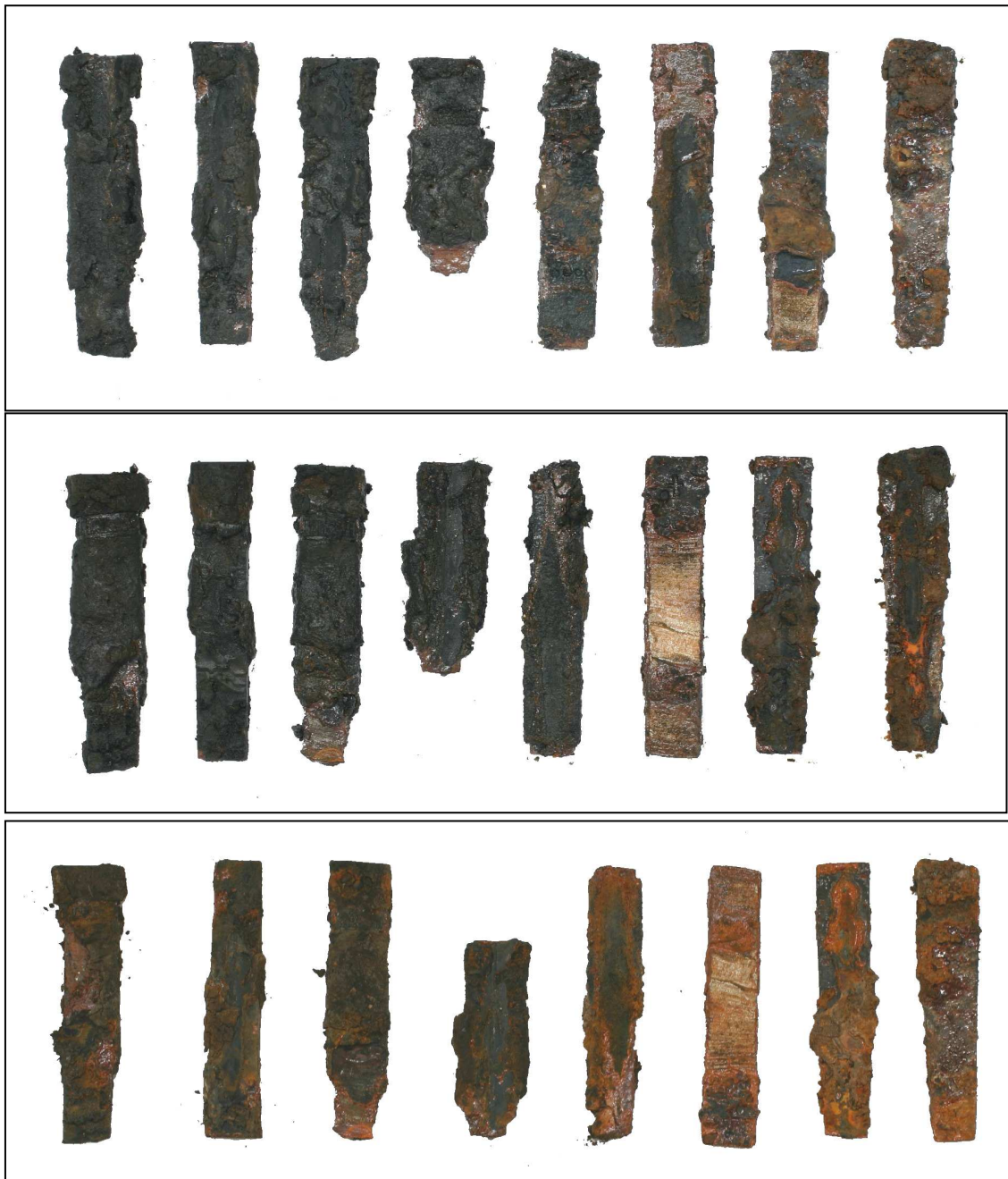
Figure 7. Cluster 2 coupons as recovered showing the variability in condition and colour. The top two rows show the two sides of the same eight bars, in sequence with coupons 1 at the left, coupon 8 at the right. The coupons have been removed from the installation rod and loose soil has been detached, but they have not yet dried out. The lowest row shows one side of the coupons after being dried out (the sequence across the page is the same as in the upper two rows but their orientations are not necessarily the same). Lengths of original coupons c. 50mm.
