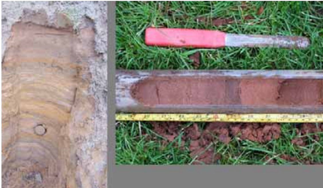
Figure 2: OSL sampling from exposures at Brockholes gravel pit (right); and (left) typical sands targeted for OSL dating that predominantly are reworked Permo-Triassic bedrock
