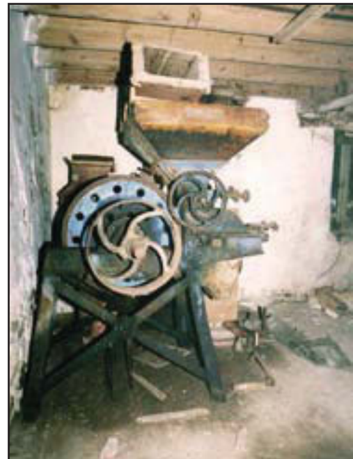
Figure 23. Interior, first floor of mill, from east, showing the oats crusher in the north-east corner. [OP04340]
