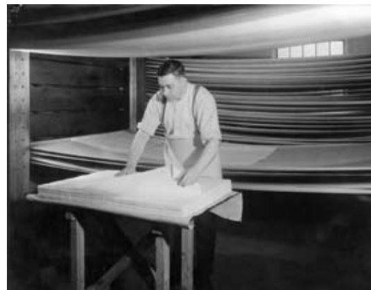
Figure 45: Undated, c.1950s photograph of the drying loft on the first floor of Building 21. (Photograph supplied by Nick Pearson).
