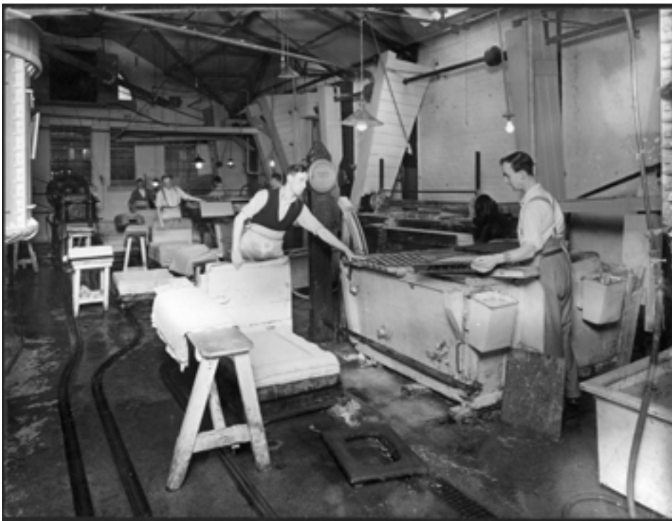
Figure 29: A century on, vatman and coucher still at work in Building 5, although Donkin's machine is gone (undated c.1950s photograph supplied by Nick Pearson).
