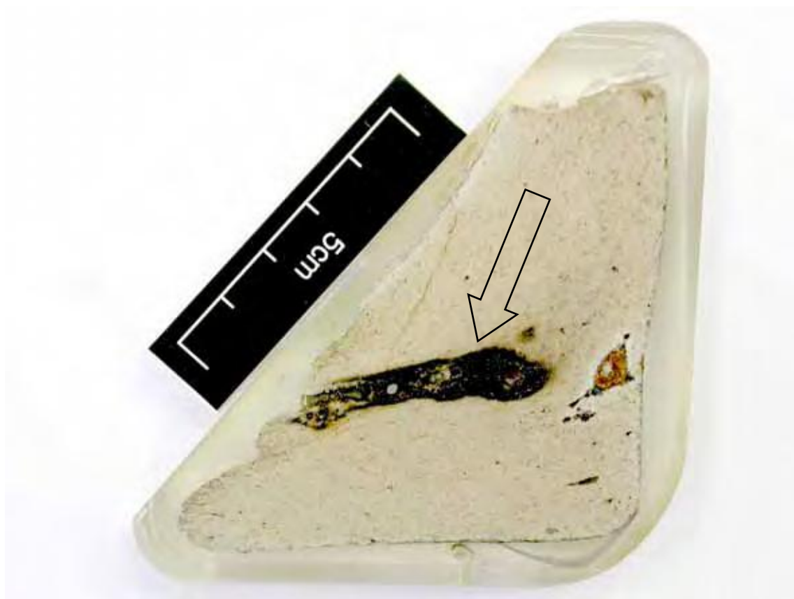
Figure 8. Crucible #28 showing the vitrified zone between the base and wall
