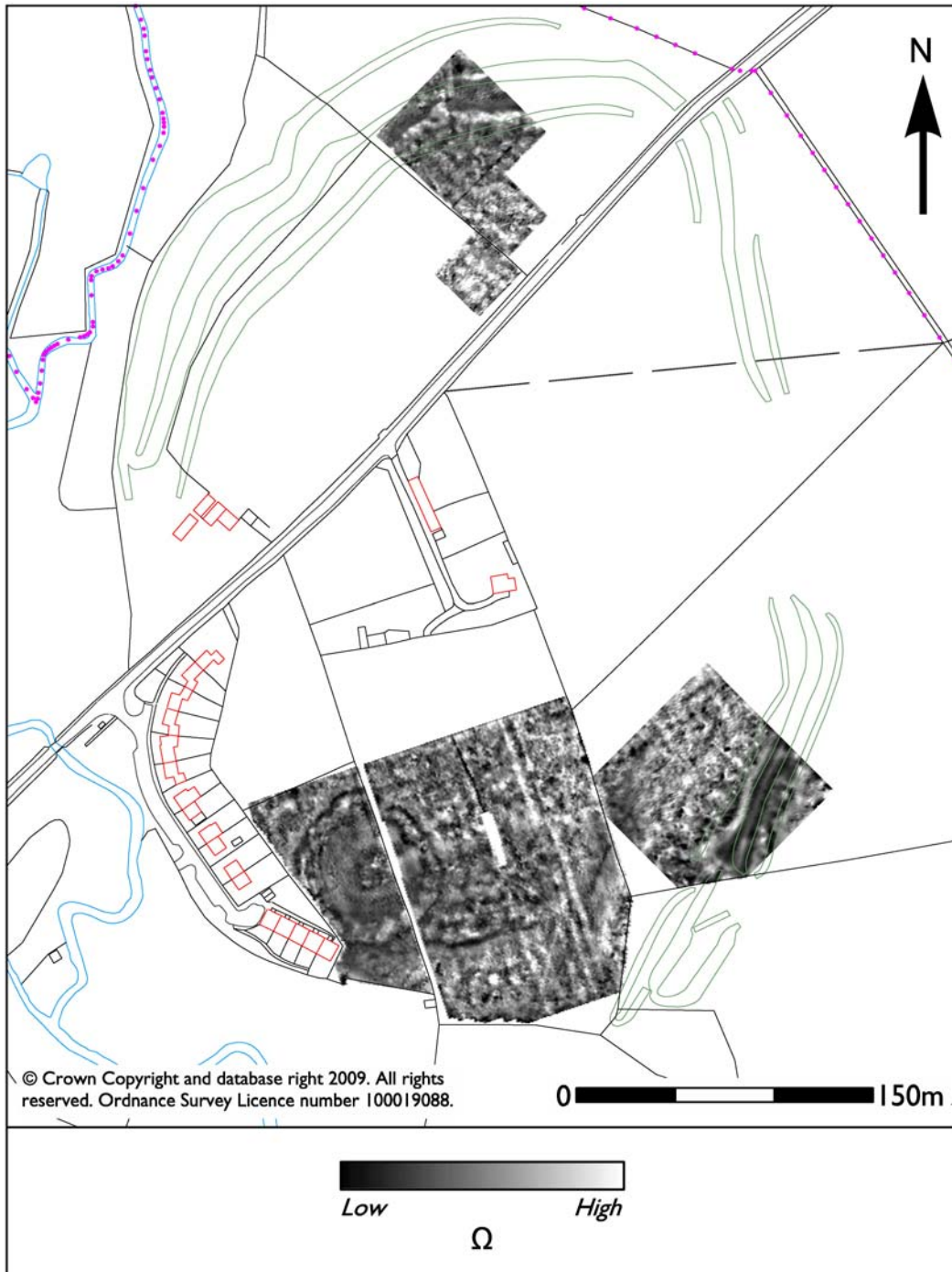
Figure 18 Twin probe earth resistance survey.
