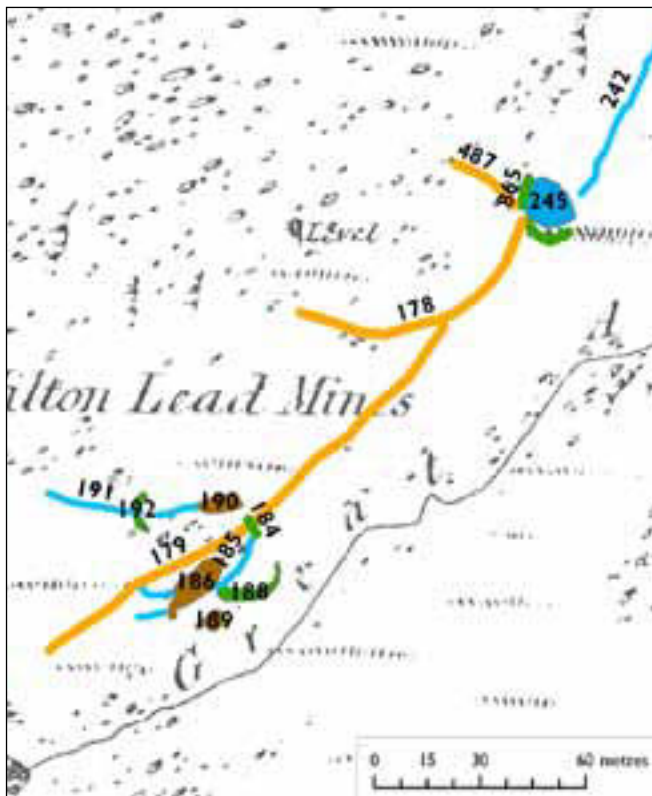
Figure 32 Extract from the GIS showing features to the north of Great Augill. The linear features shown in orange are hush channels.
