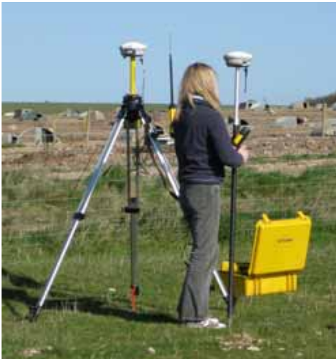
Fig 17: Calibrating the base station and configuring the roving GPS receiver
