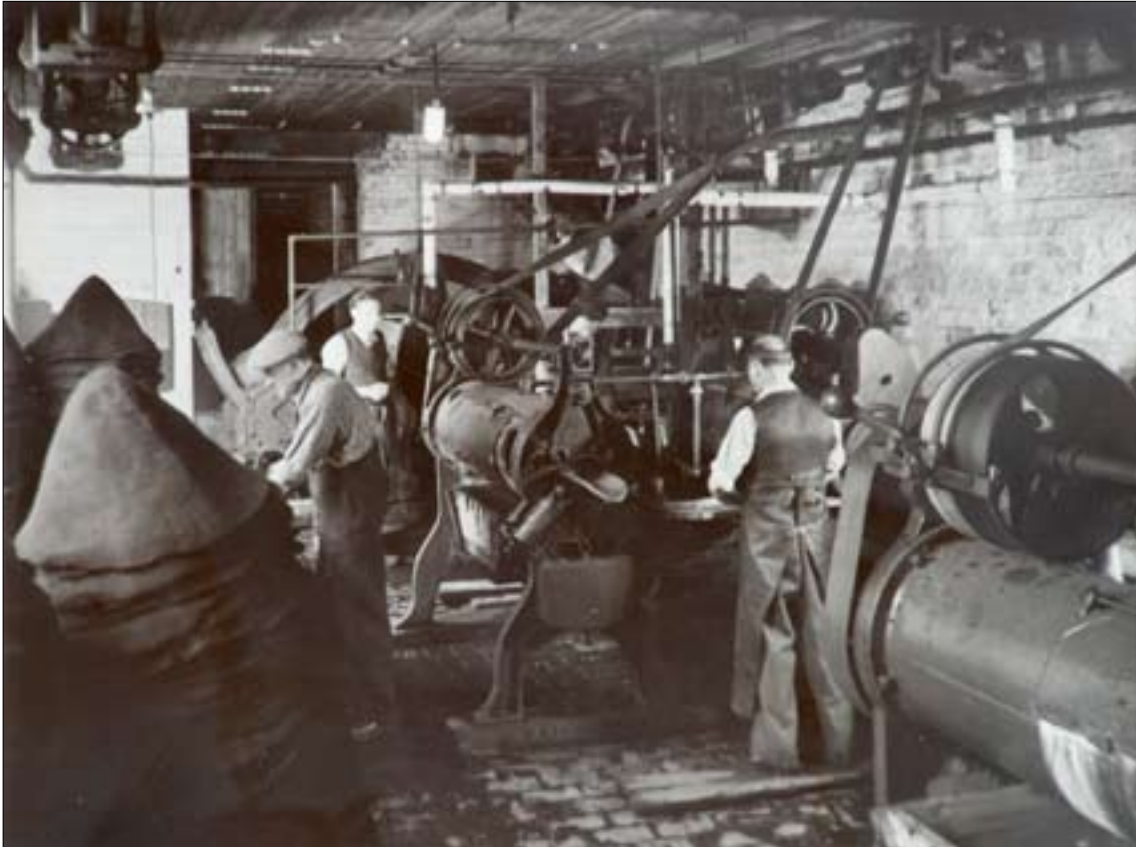
Figure 13 Rotary proofing machines for stiffening felt hoods, circa 1940. Unidentified location. Collection of Mr John Horn.
