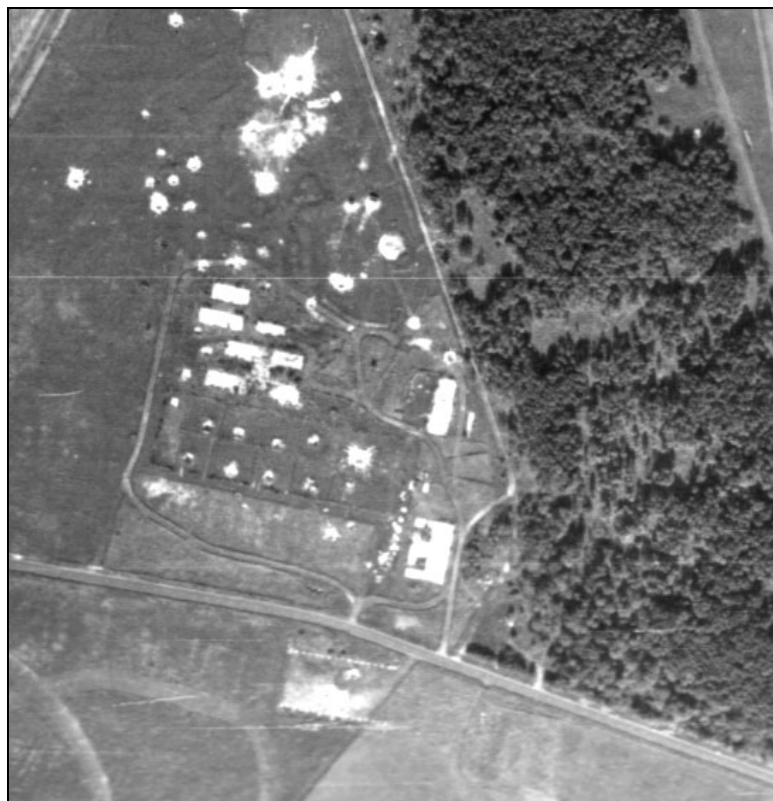
Fig 12: The pig farm and demolished Night Camp in 1945. The larger white rectangles are the highly reflective concrete bases of the Night Camp buildings. The footings of the First World War hangars and other associated structures are visible south of the road. NMR RAF/106G/UK/915 extract from frame 4205 11th October 1945. English Heritage (NMR) RAF Photography.
