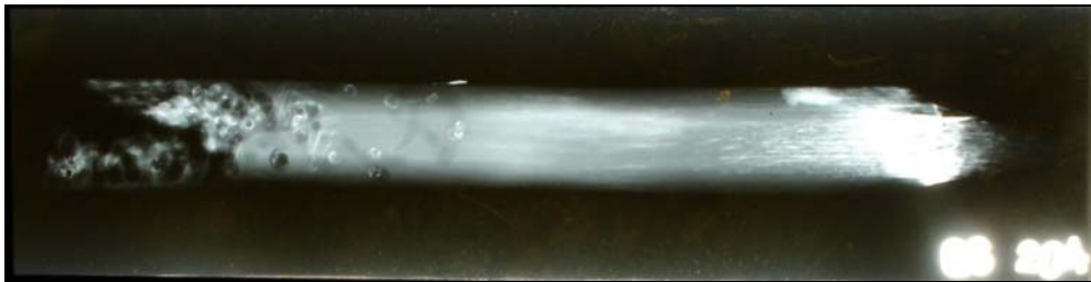
Figure 18: Pike (204) before conservation. Wood borer activity visible in X-radiograph
