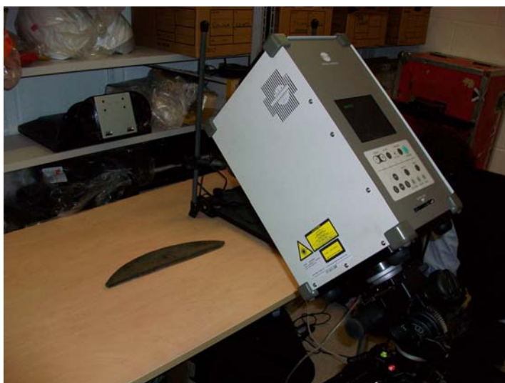
Fig 11: Laser scanning of the post-conservation timber
