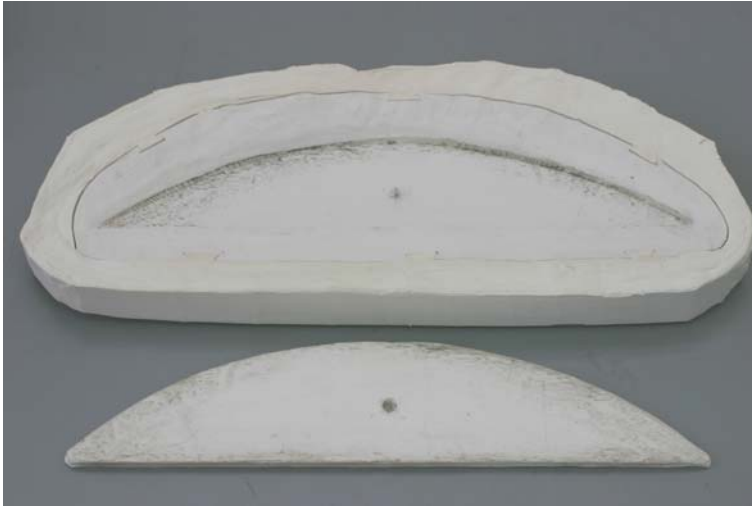
Fig 10: Silicone mould and plaster of Paris cast
