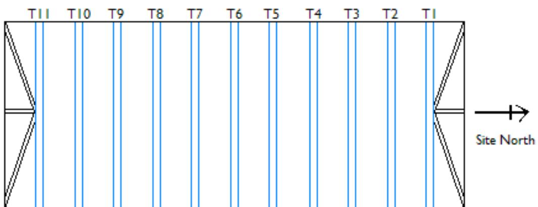
Figure 43: Threshing barn; sketch plan of first floor, showing the location of roof trusses
