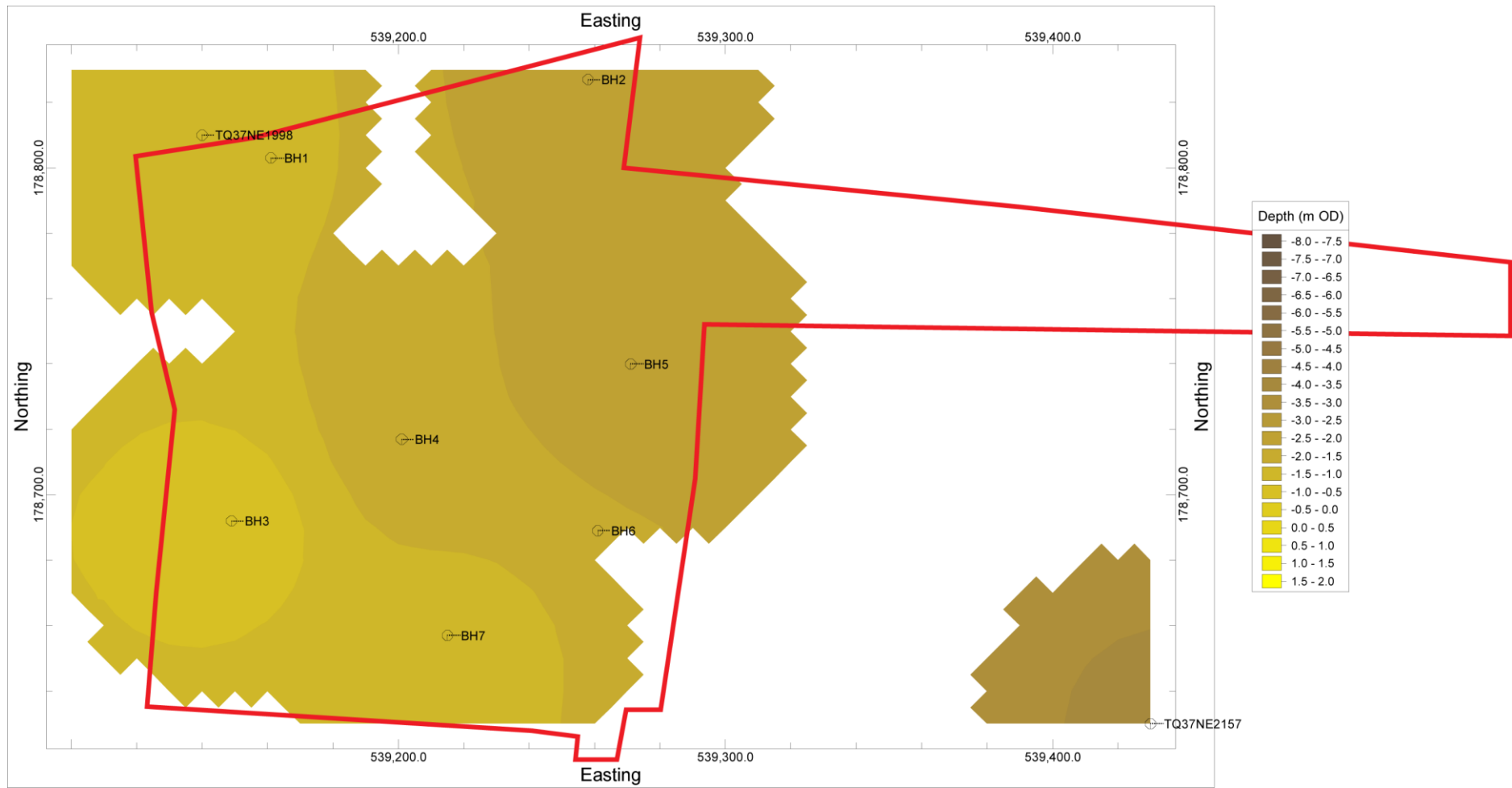
Figure 4: Modelled surface of the Lower Alluvium (contour heights in metres OD).
