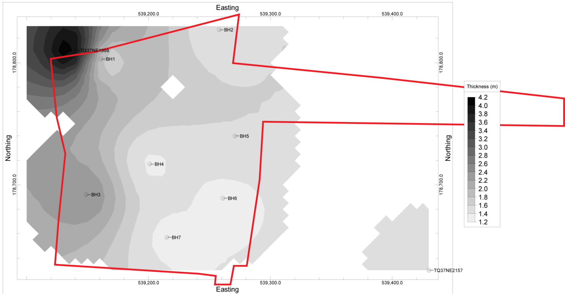
Figure 9: Modelled thickness of the Made Ground (metres)
