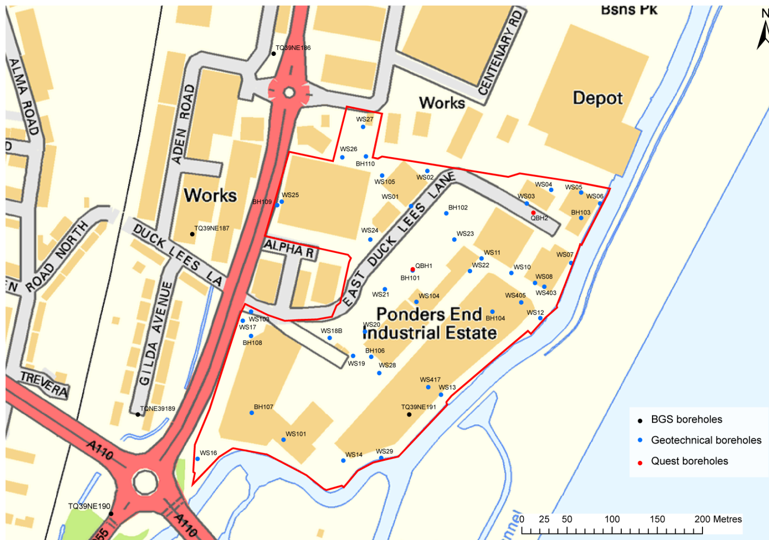
Figure 2: Location of the new geochronological (red) and geotechnical boreholes (blue), and existing BGS borehole records (black) at Enfield Distribution Park. Contains Ordnance Survey data © Crown copyright and database right [2012].
