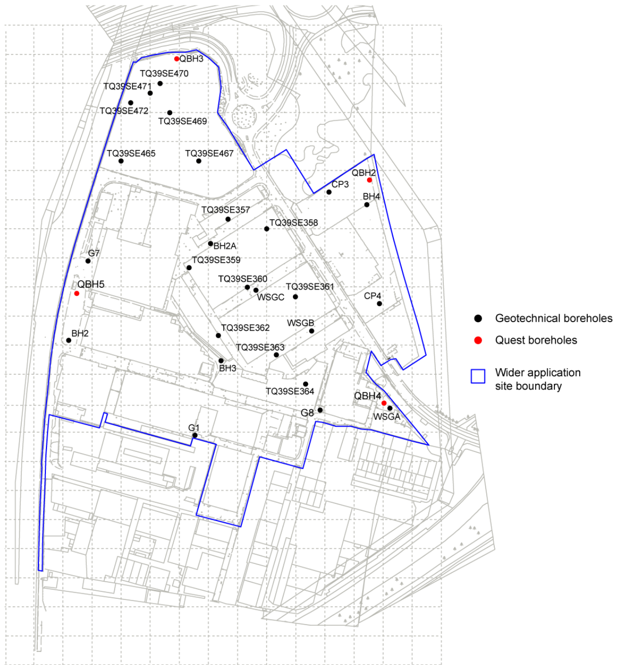
Figure 2: Location of the new geoaerchaeological (red) and existing geotechnical (including BGS records ( www.bgs.ac.uk/opengeoscience ) boreholes (black) used in the deposit model at Stonehill Business Park. Original figure provided by CgMs Consulting.
