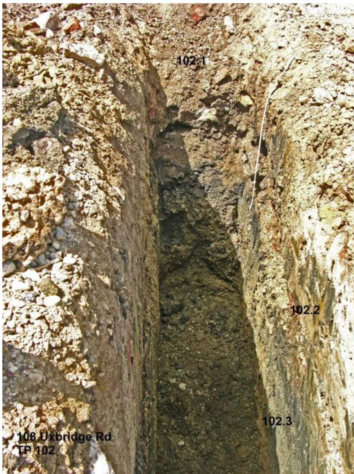
Figure 6: Trial pit TP102, annotated photograph.
