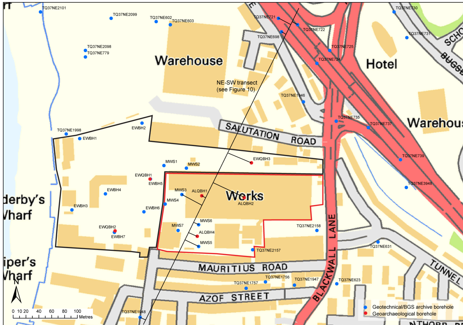
Figure 2: Location of the new geoarchaeological boreholes at the Alcatel Lucent Telegraph Works site (red outline) and existing geoarchaeological, geotechnical and BGS archive boreholes in the area of the deposit model, including those at Enderby Wharf (Batchelor et al., 2015a; black outline). Contains Ordnance Survey data © Crown copyright and database right [2012].
