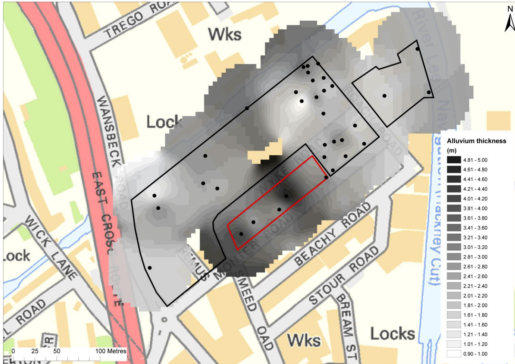
Figure 8: Thickness of Alluvium (m) (site outline in red). Contains Ordnance Survey data © Crown copyright and database right [2016].
