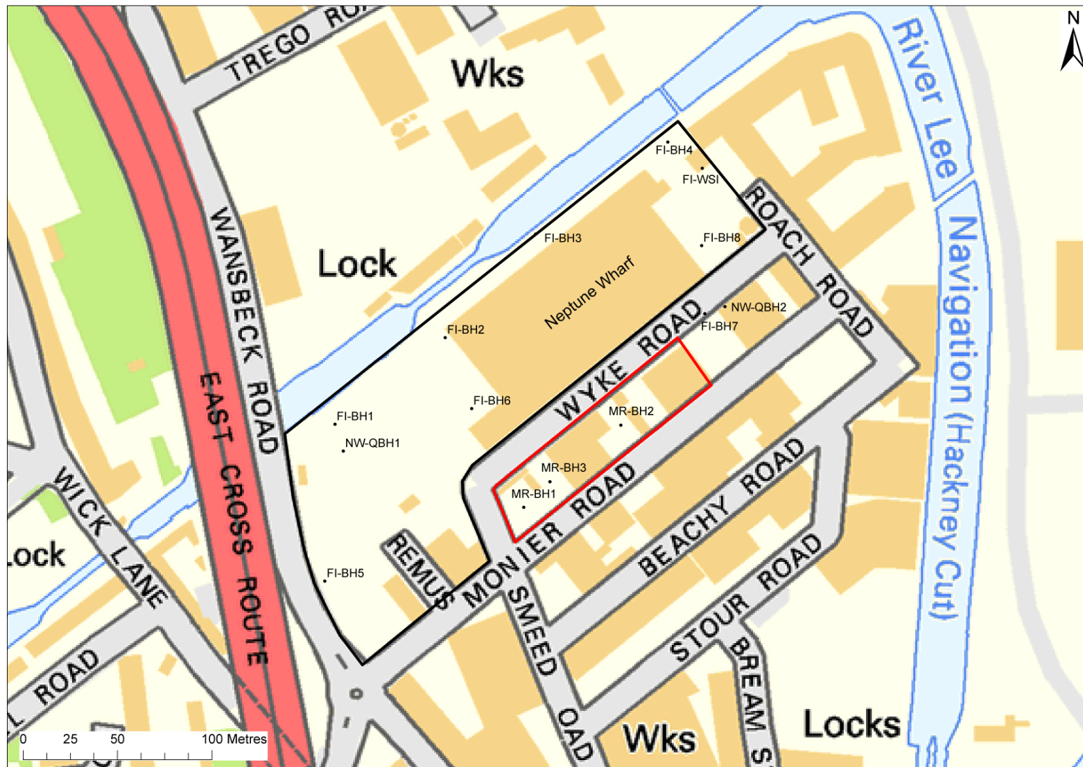
Figure 2: Location of the geotechnical and geoarchaeological boreholes at the 79-85 Monier Road site, London Borough of Tower Hamlets
