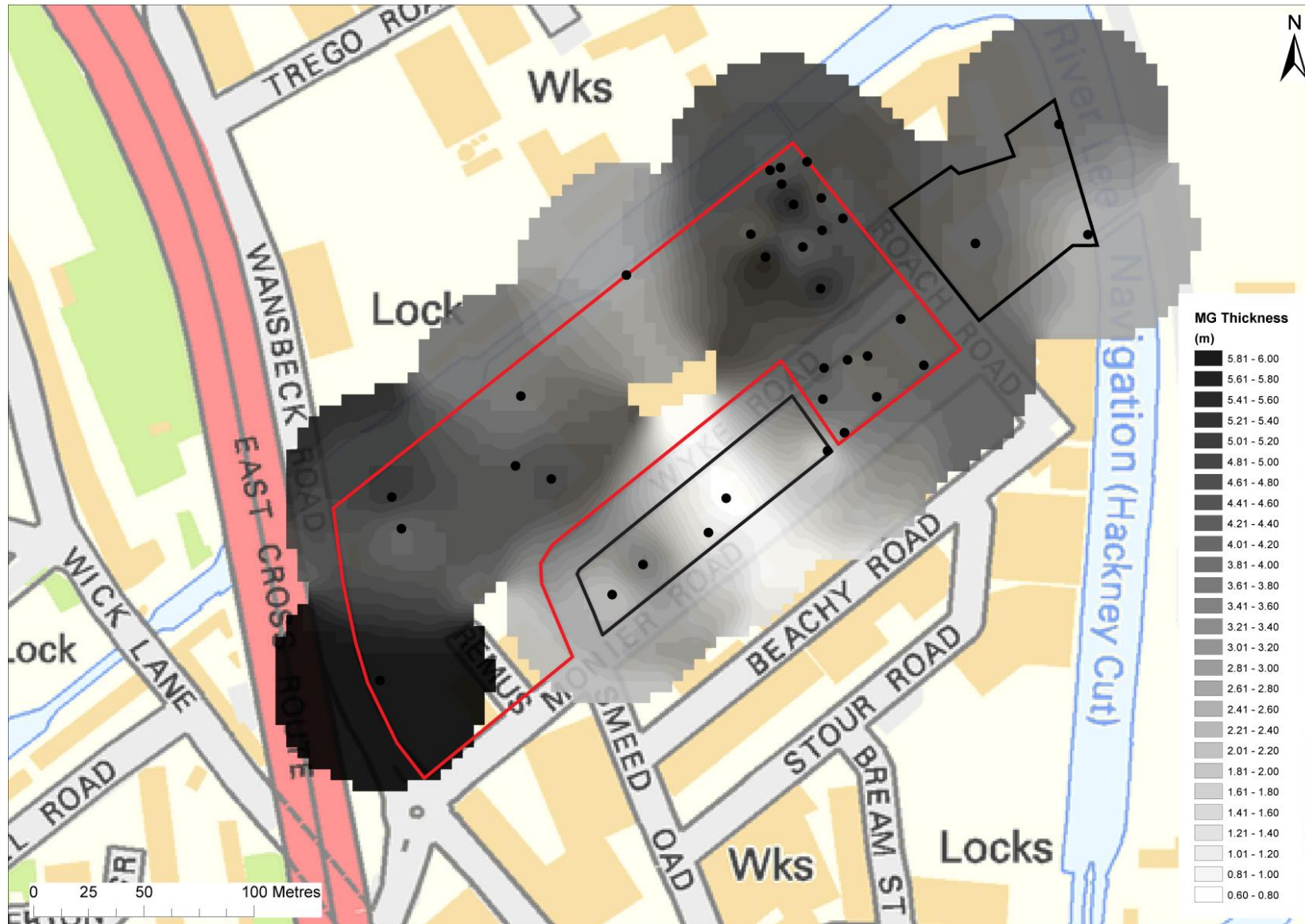
Figure 9: Thickness of Made Ground (m) (site outline in red). Contains Ordnance Survey data © Crown copyright and database right [2016].
