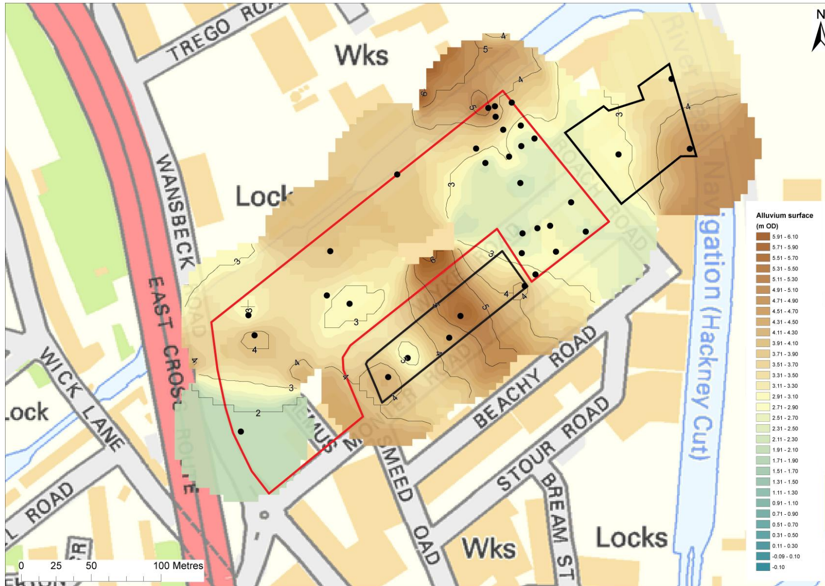
Figure 7: Top of the Alluvium (m OD) (site outline in red). Contains Ordnance Survey data © Crown copyright and database right [2016].
