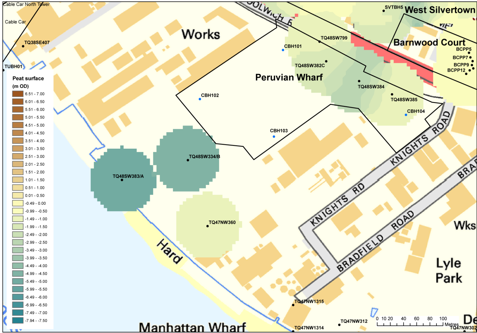
Figure 6: Modelled surface of the Peat (m OD)
