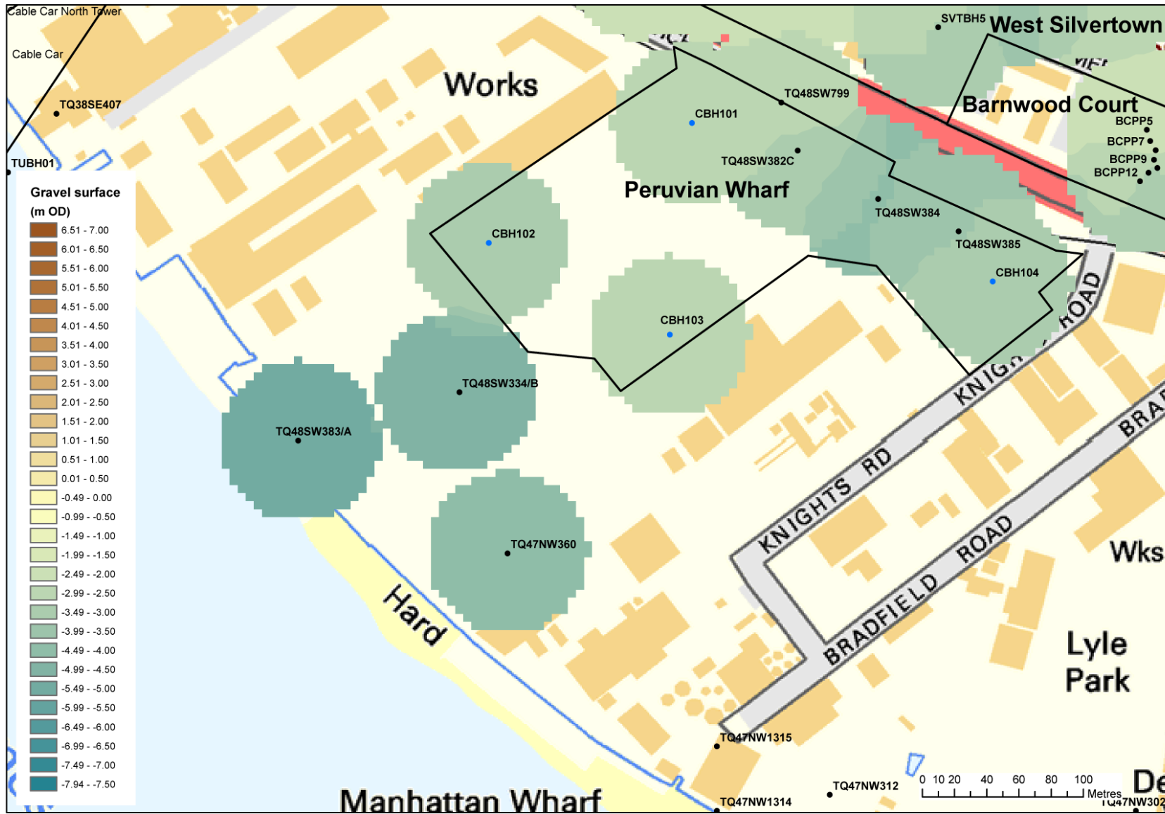
Figure 5: Modelled surface of the Shepperton Gravel (m OD)
