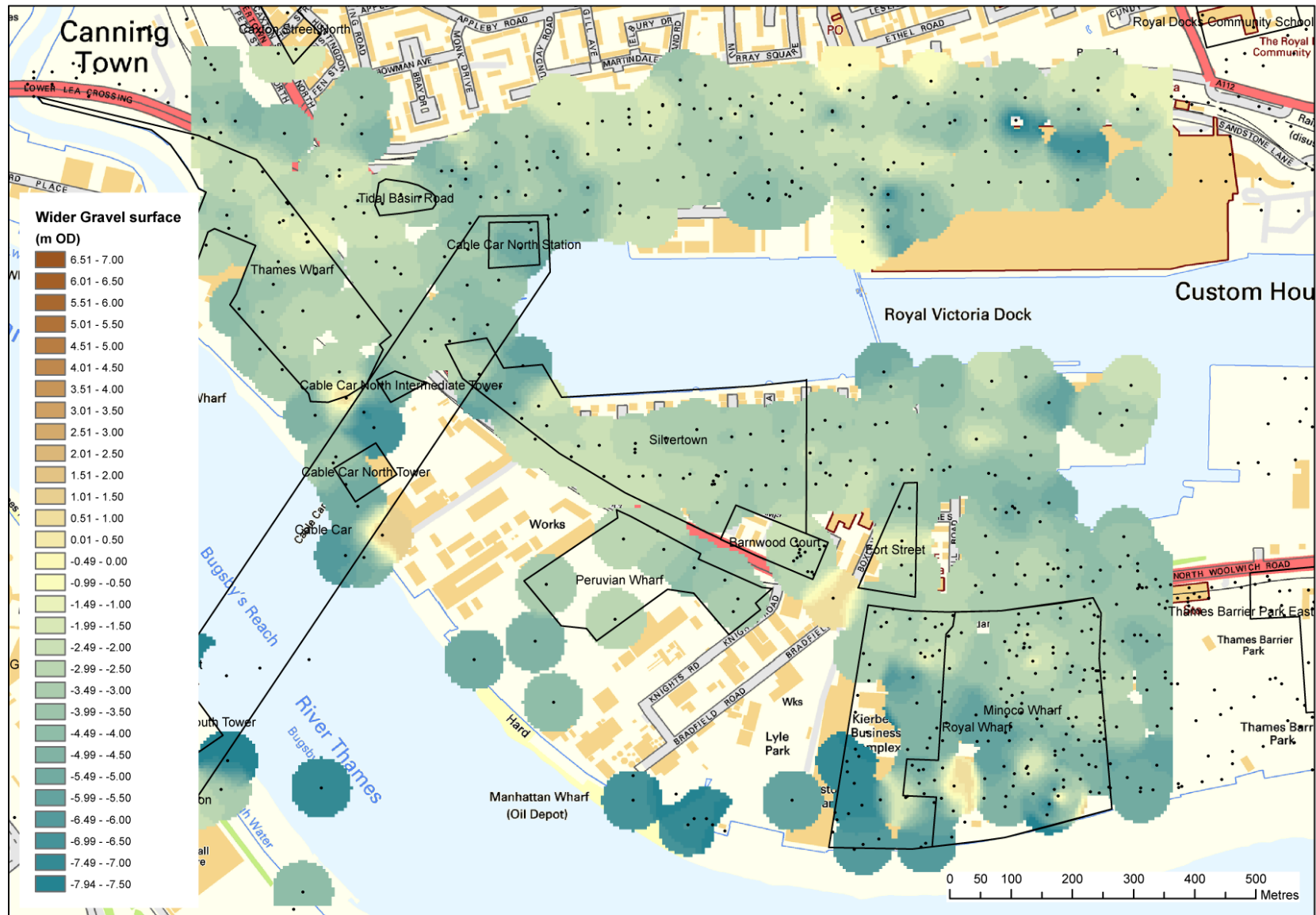
Figure 11: Modelled surface of the Shepperton Gravel (m OD) across the wider area
