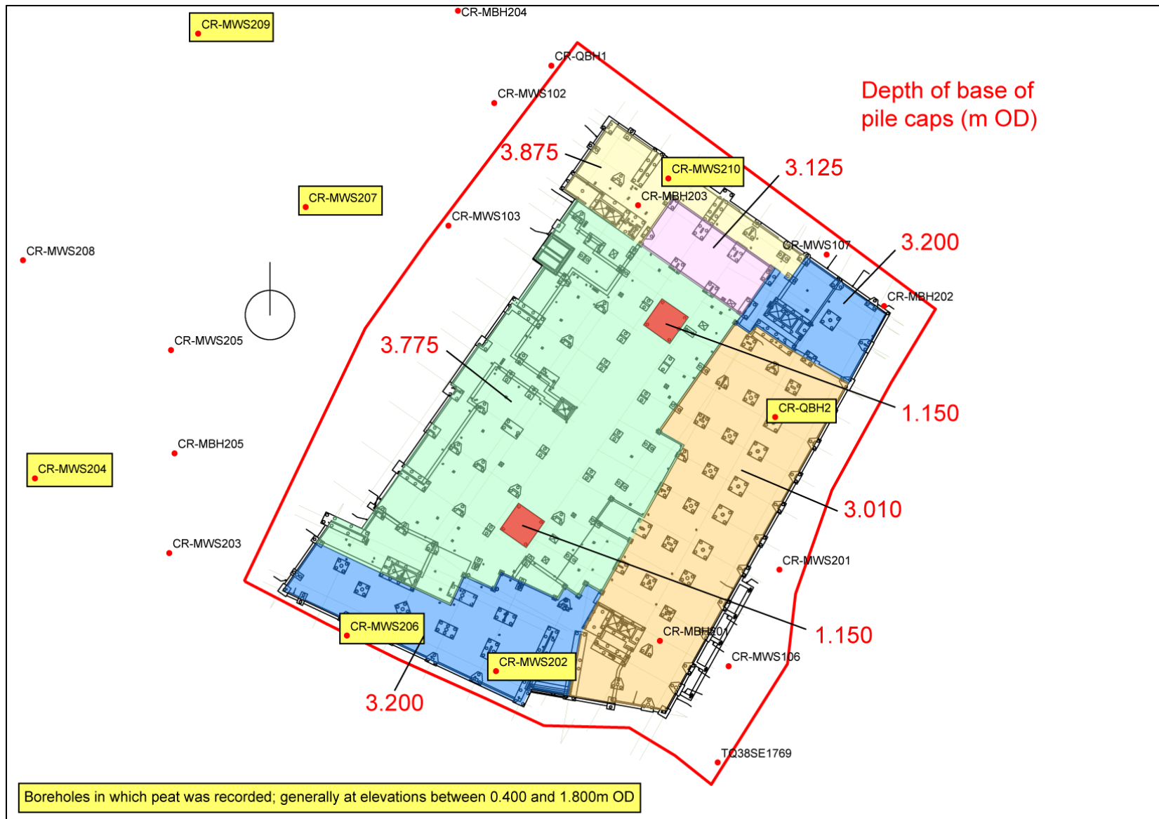
Figure 12: Impact of the pile caps at the Cooks Road Block B site.
