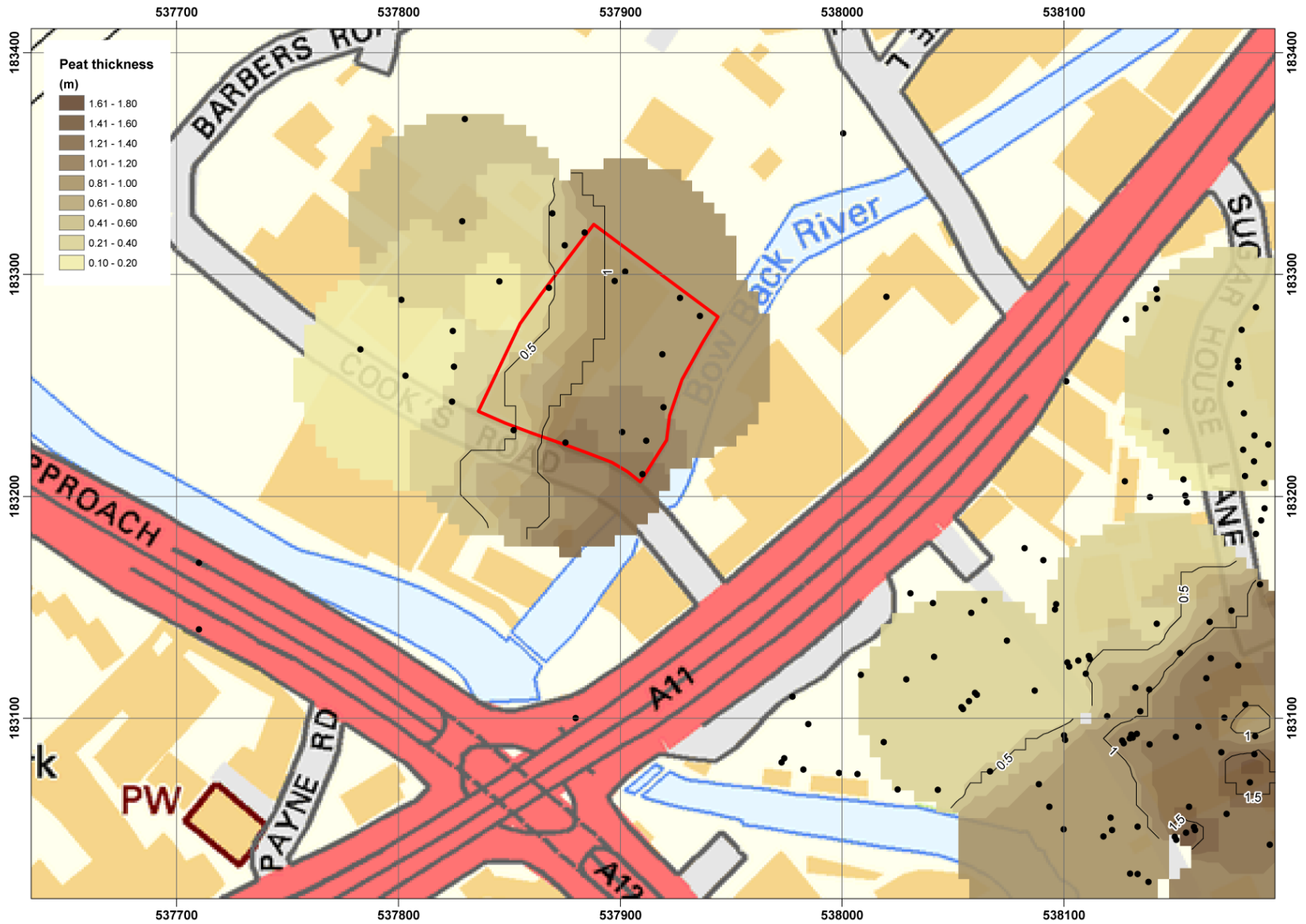
Figure 6: Peat thickness (contour heights in m). Contains Ordnance Survey data © Crown Copyright and Database right 2016.
