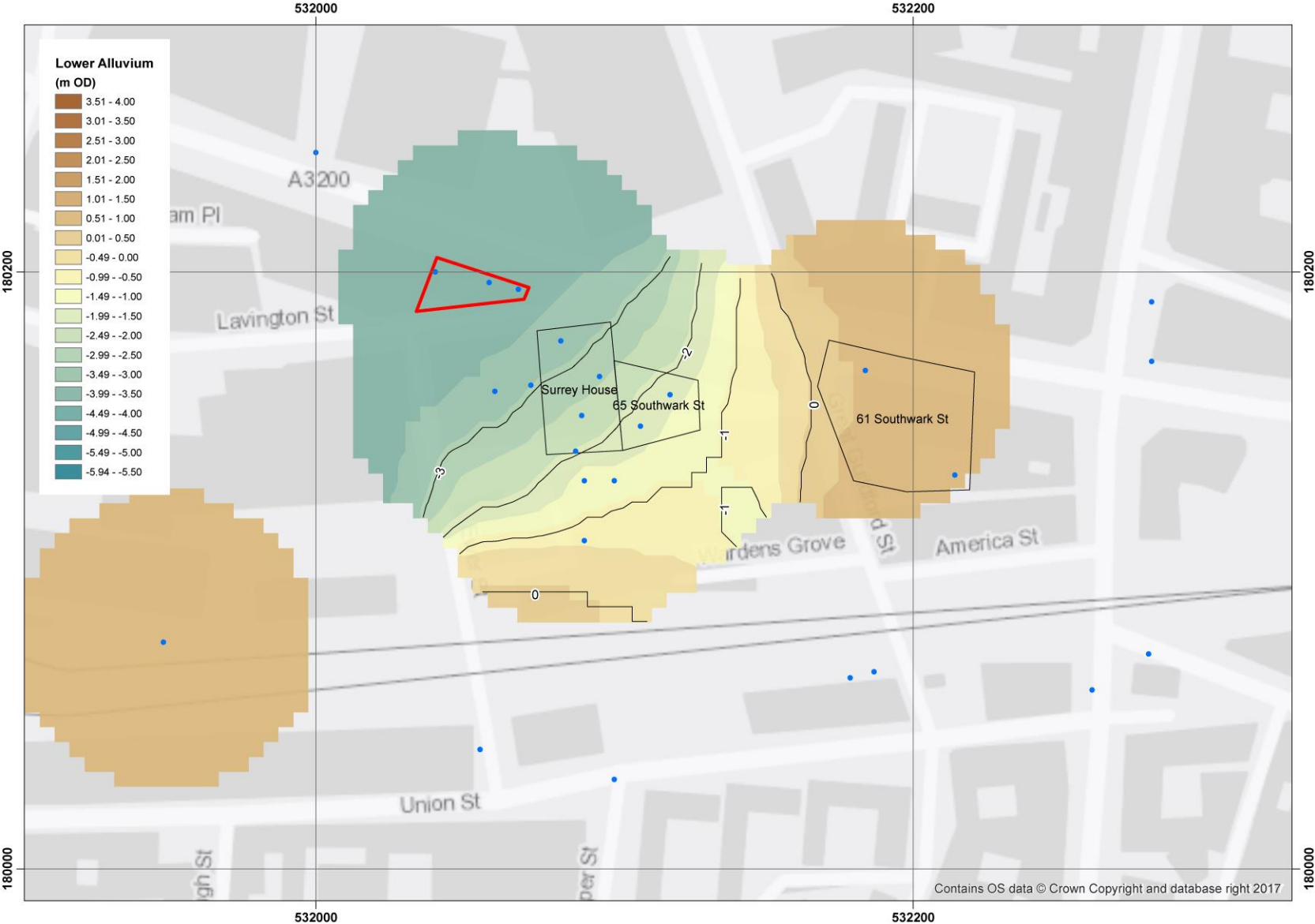
Figure 5: Top of the Lower Alluvium (m OD) (site outline in red).
