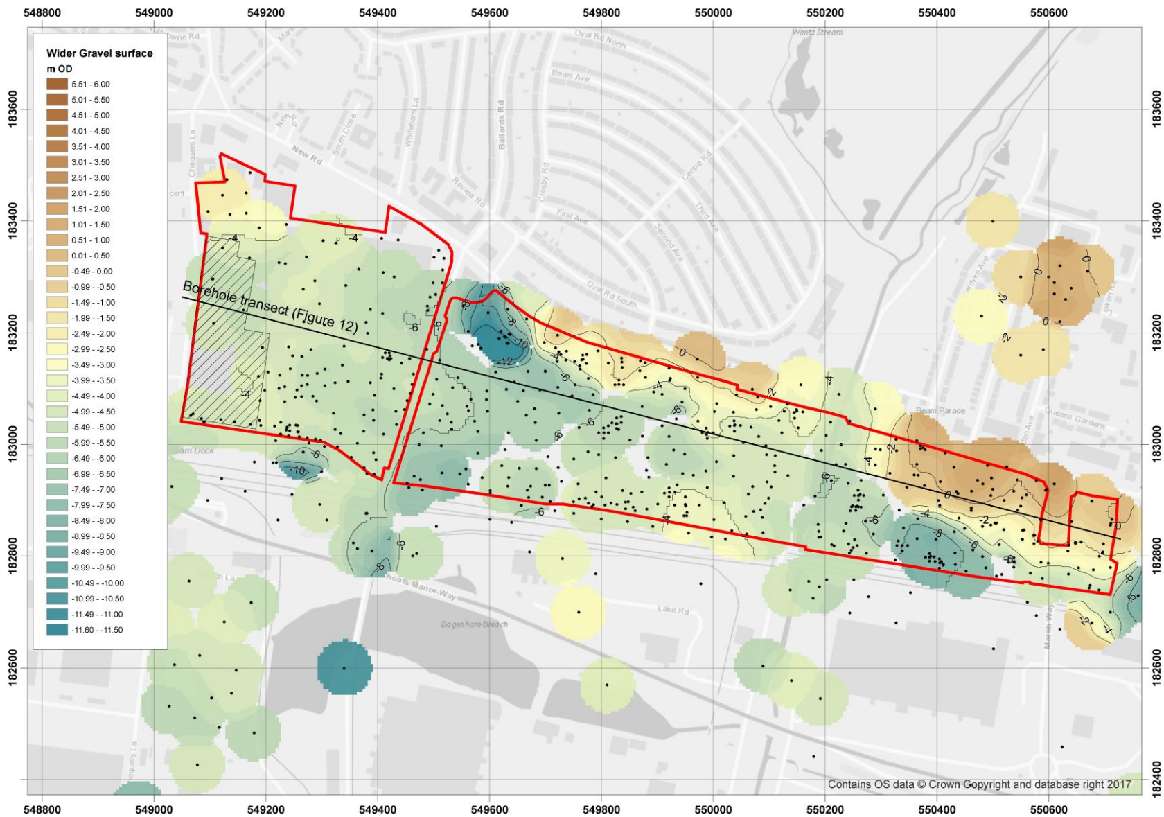
Figure 4: Top of the Gravel across the wider area (m OD) (site outline in red)
