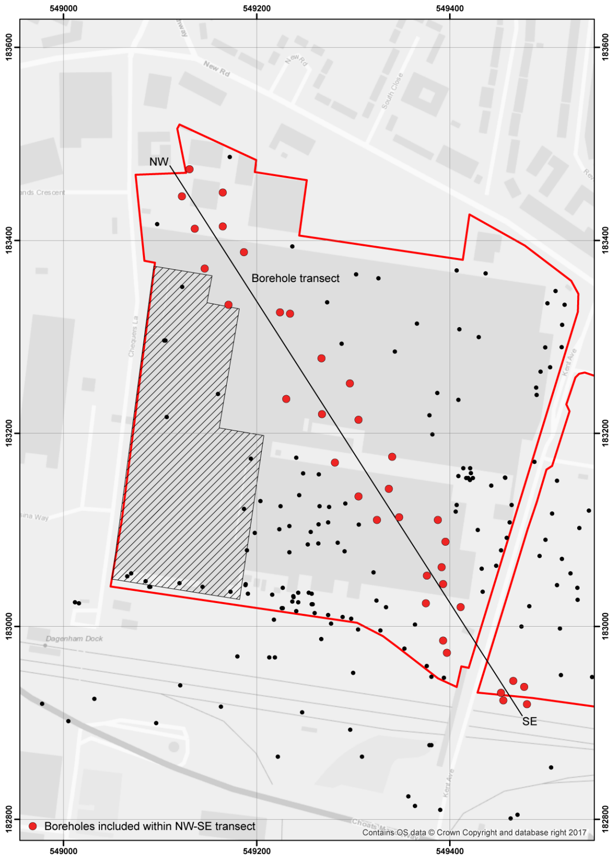
Figure 2: Location of boreholes across the Former Ford Stamping Factory site.
