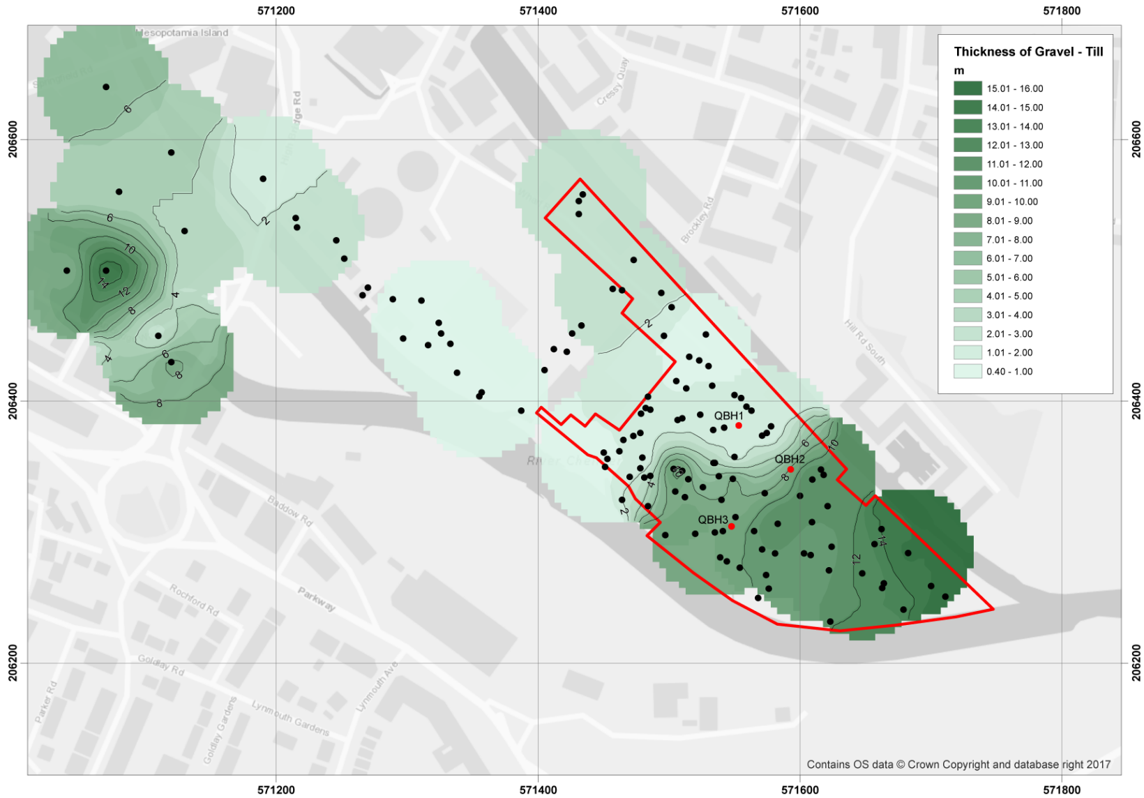
Figure 3: Combined thickness of the MIS12 Chalky Till / Gravel and late Devensian / early Holocene River Chelmer Gravels (m), showing SI borehole and test-pit locations (black) and the new geoarchaeological boreholes (red).
