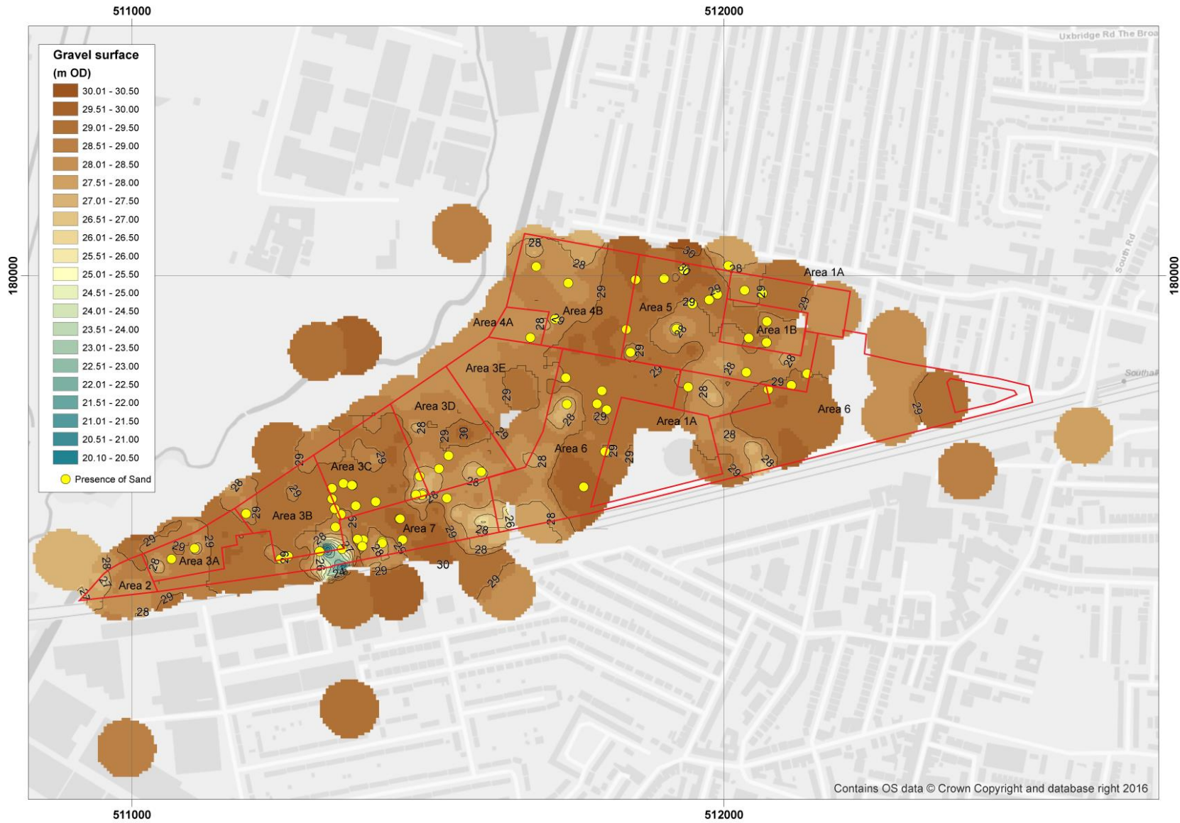
Figure 4: Top of the Lynch Hill Gravel (m OD); sequences including the presence of sand are highlighted in yellow
