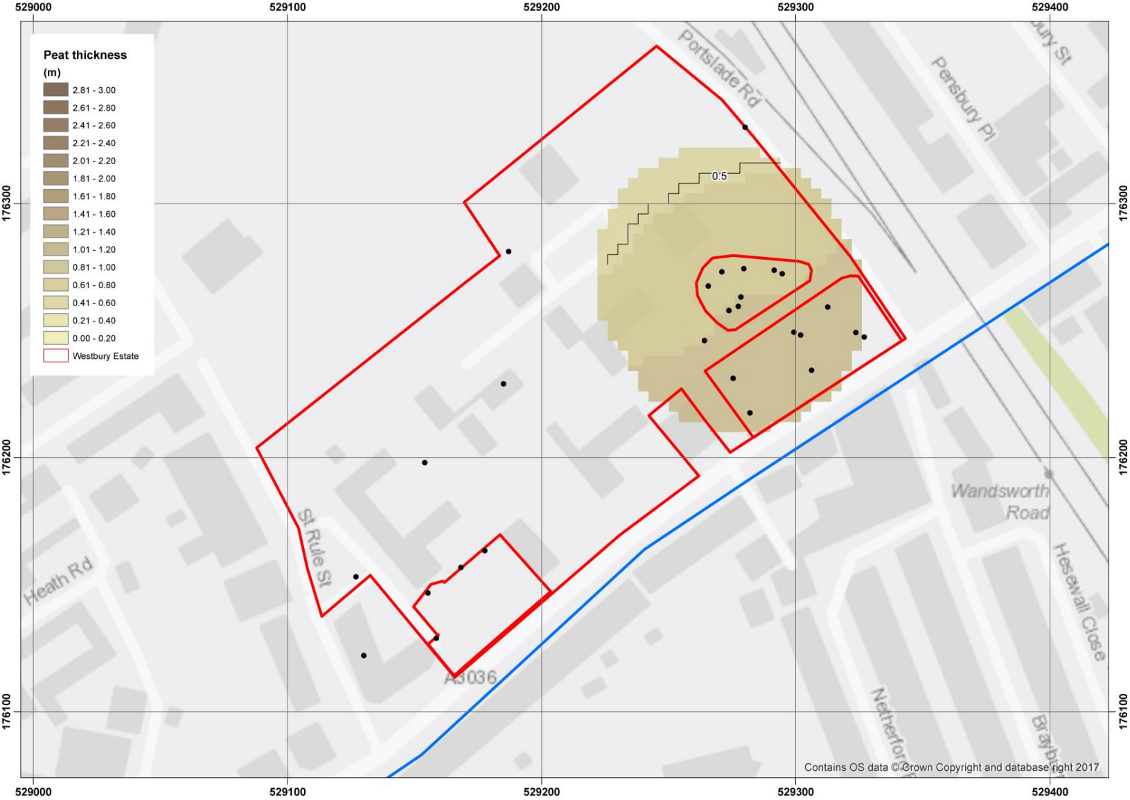
Figure 8: Peat/Organic Clay thickness (contour heights in m).
