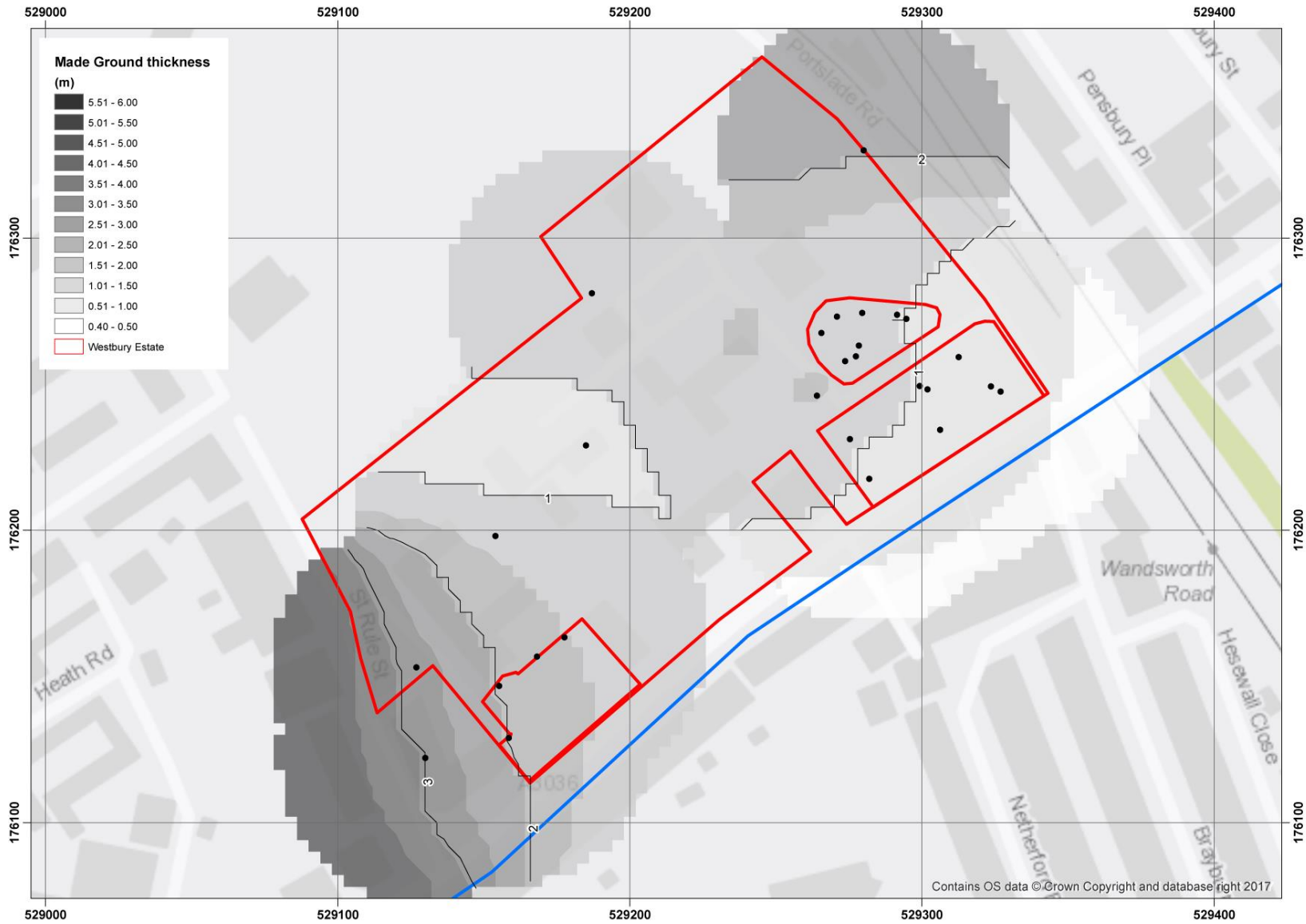
Figure 11: Made Ground thickness (contour heights in m).
