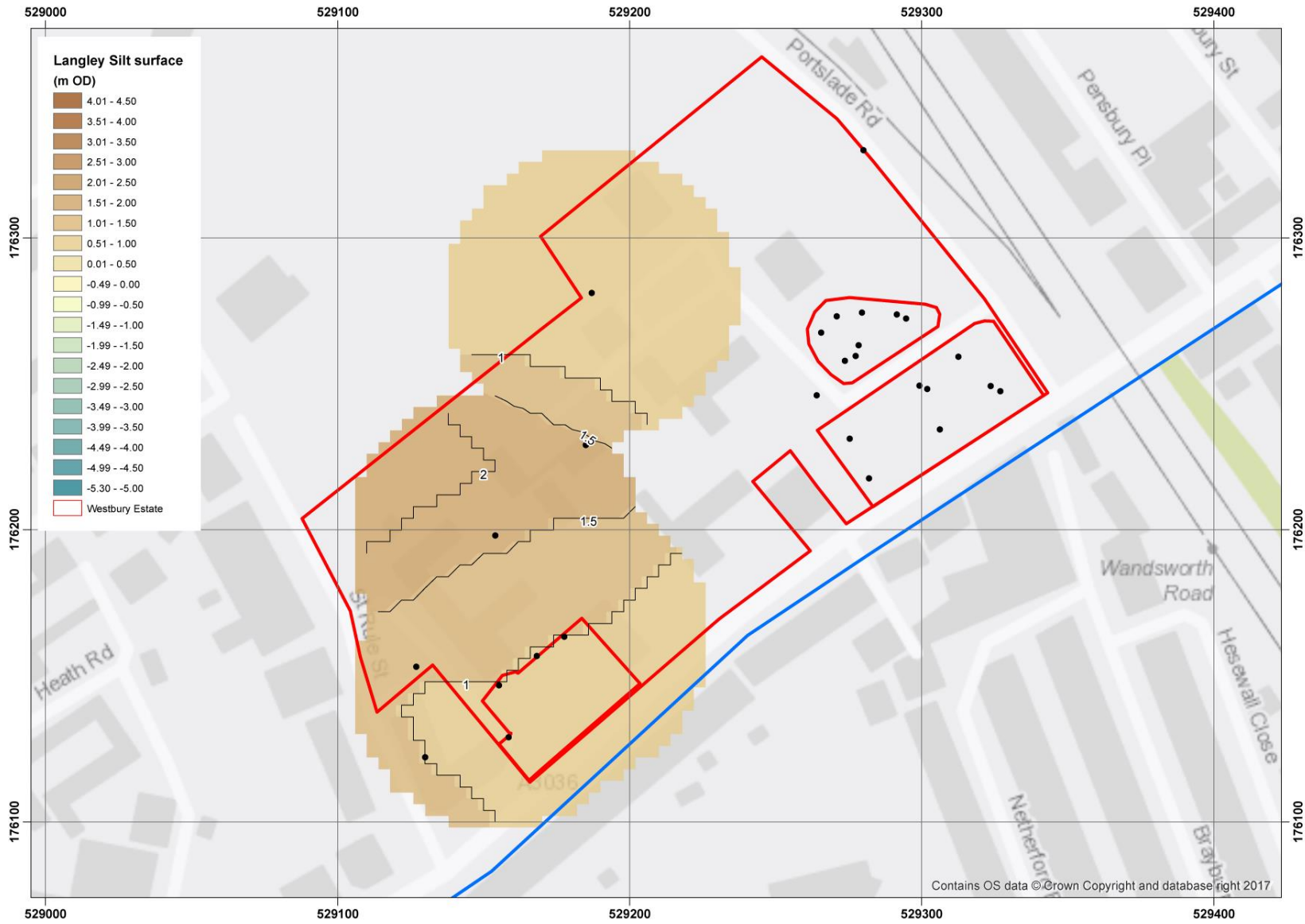
Figure 5: Langley Silt surface (contour heights in m OD).
