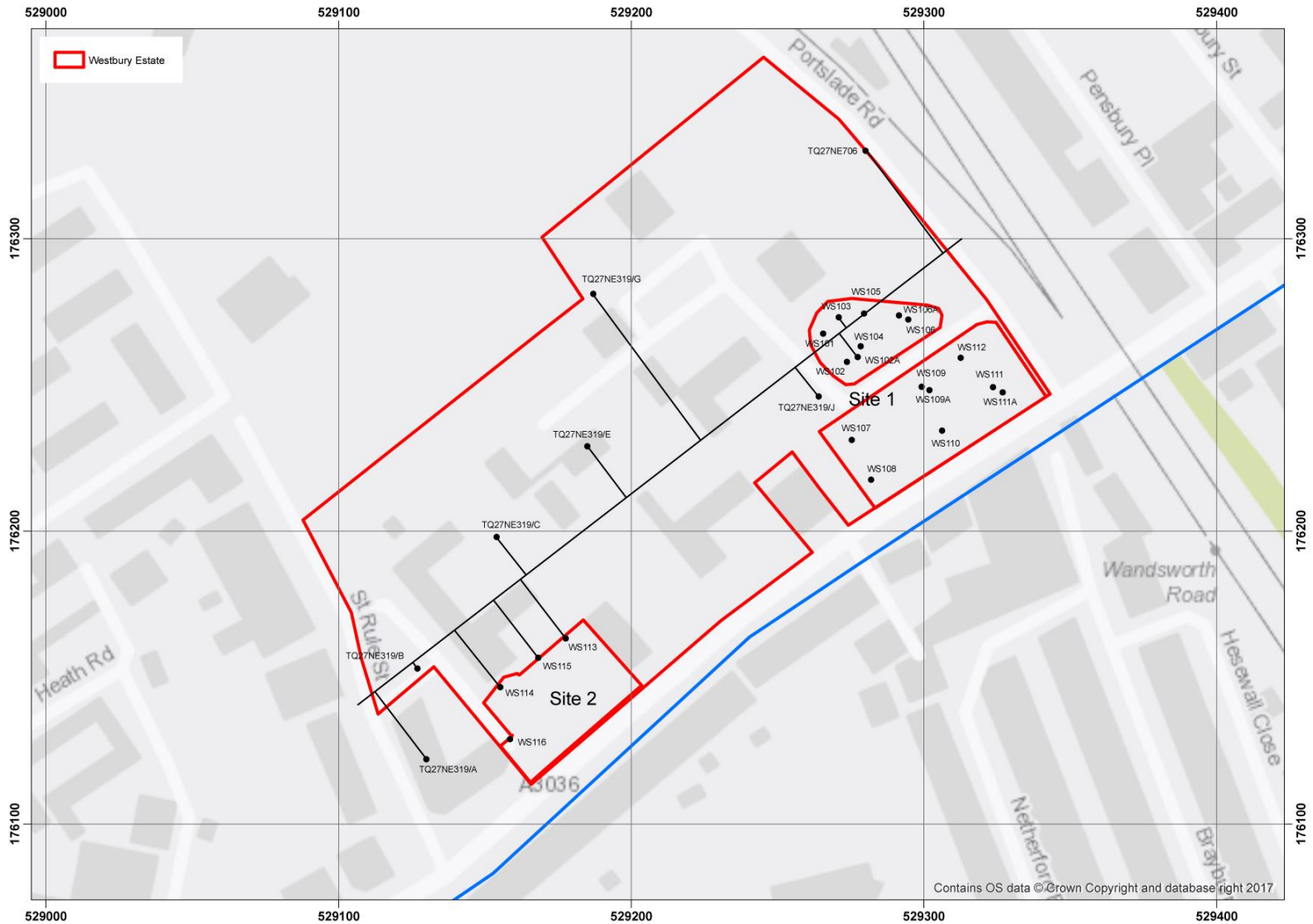
Figure 2: Location of the boreholes used in the deposit model at the Westbury Estate, Wandsworth Road, London Borough of Lambeth. Orientation of the southwest-northeast transect also shown (see Figure 12).
