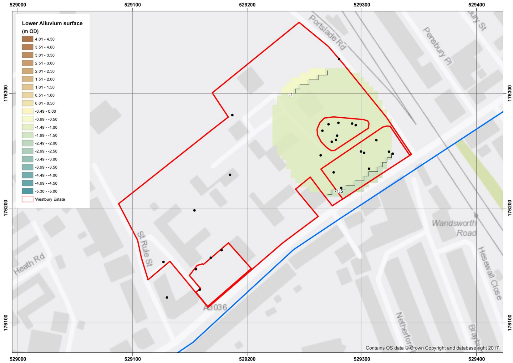
Figure 4: Lower Alluvium surface (contour heights in m OD).
