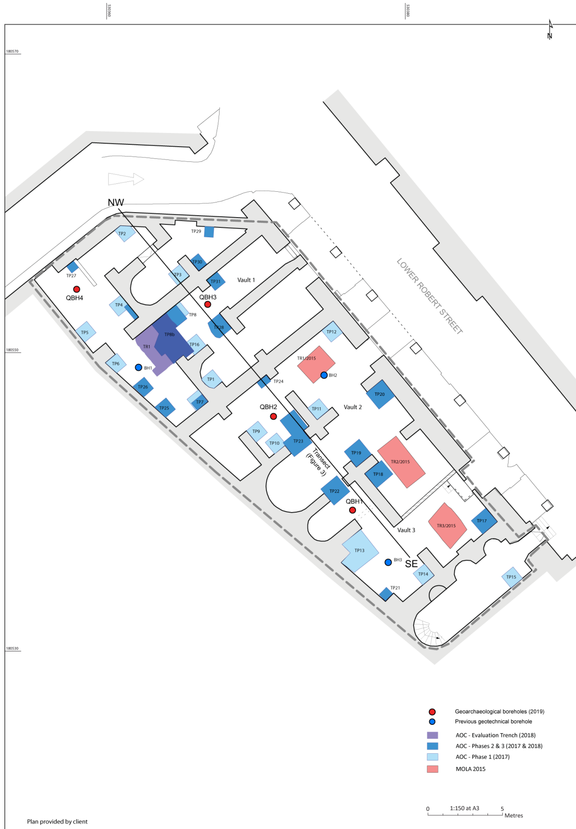
Figure 2: Location of the new geoaerchaeological boreholes (QBH1 to QBH4), and previous previous archaeological/geotechnical interventions carried out by MoLA (2015), AOC (2017), AOC (2018a) and AOC (2018b) at 2-3 Robert Street, London Borough of Westminster. Figure adapted from AOC (2018b). Orientation of NW-SE transect (see Figure 3) also shown.
